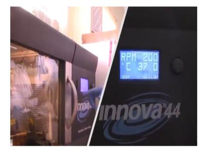
So, the machine that I have in front of me now is a temperature control shaker incubator and the purpose of this is that it allows us to grow bacteria in a controlled temperature environment. As you can see inside there are different flasks containing volumes of bacterial growth media, in which bacteria have been inoculated and as time progresses, they will grow in a temperature controlled environment.
