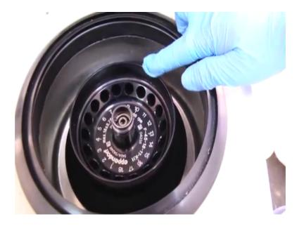
So, as you can see these small holes, inside these holes we can play small eppendorf tubes and right now the machine is switched off, but what will happen is once I put the centrifuge tubes here the machine rotates. And as you can see the centrifuge tube which has been placed here or which will be placed here will always remain at a constant angle.
