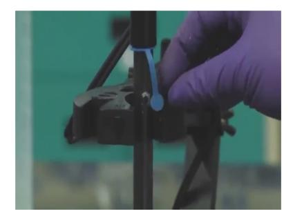
So, in order to do the pH meter calibration, first I will take out the probe from the storing solution and as I mentioned earlier, before you dip the probe in any solution you have to
