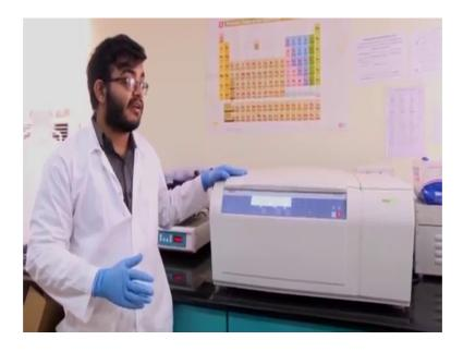
What I have in front of me now is a centrifuge, it is a temperature control centrifuge and its purpose is to centrifuge different samples. And this is a temperature control centrifuge, which means we can maintain it at 25 degree centigrade or lower 24 degrees or 16 degrees or even if required slightly higher.
