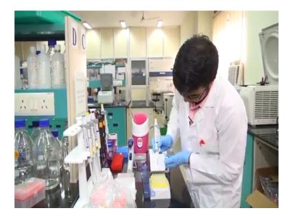
I was also talking about the multi-channel pipette. Remember which can use this one can use eight tips at a single go. Suppose I want to collect 100 micro liters, 8 times instead of doing it 8 times, I can do it in one go in which case you align the nozzles with the tips you press down slight motion and see you actually have volumes here.
