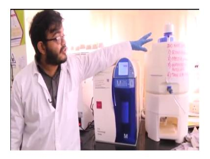
And finally, the purified de ionized water that is present is stored in this tank from which we can take as per our requirement.
