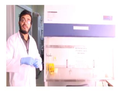
So, this instrument is a laminar air flow cabinet and you will be looking at this instrument later on in further detail in the subsequent lectures, but in general what this instrument is used for, is basically once you open this and it is switched on. There is an
