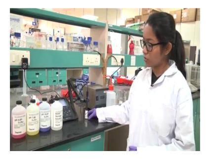
So, now theat I have already mentioned you about the pH meter. So, this is a digital pH meter and the probe should be always kept inside the solution storing solution.
