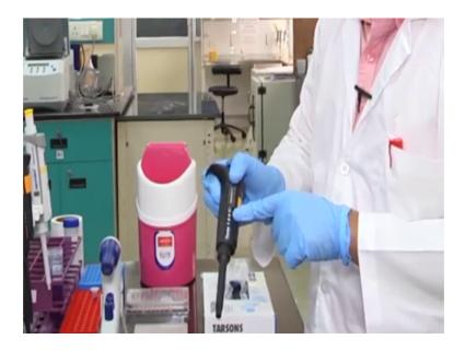
When you are done working with the pipette, always keep it in its released condition. The released condition corresponds to the maximum volume that can be pipe it pipette, it out with that instrument.
