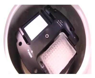
For many type of experimental purposes you might need to centrifuge samples kept inside 96 well plates and for that purpose, this sort of centrifuge rotor is necessary.
