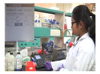
Now I am using a standard solution of page 4.0 and then I will dip this probe inside this solution. Now be very careful how much you dip the probe inside the solution. The probe should be or the bulb should be absolutely immerse inside the solution do not drip it till here otherwise this buffer might go inside your probe.
