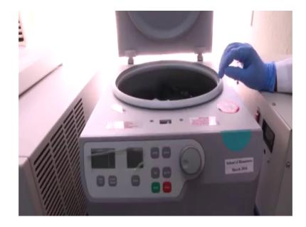
This centrifuge here has a different type of rotor. So, till now what you have seen is, centrifuge rotors which can accommodate centrifuge tubes 1.5 ml centrifuge tubes, there are rotors which can accommodate 15 ml falcon tubes or 50 ml conical falcon tubes. But this rotor that I will be showing you here is a bit different because this can actually accommodate 96 well plates.
