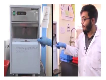
For certain experiments, it is necessary to carry out the reactions under ice cold conditions for that we need ice makers or ice flake machines. So, this small instrument here does exactly that, it is connected to a water supply source and what it does is, it creates flake ice for us; let me just show you. So, as you can see I just took out some ice. So, flaked ice, which we take inside these ice buckets and so, this is a very
