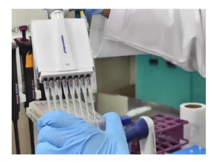
But what happens is in many aspects of molecular biology or biochemistry you will be using 96 well plates. Suppose you have to collect a particular solution from here in equal volume. At that time you dip it in here I know its empty, but I am just showing you the utility, you dip it in here, you collect the liquid and then you dispense it somewhere else and once its done you eject all the tips simultaneously.
