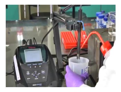
Hello today I will show you how to use a pH meter and how to measure on the pH of a solution. So, for that we have a pH meter here and in this monitor you can see the pH reading also the temperature and the volt. And along with the monitor, we will have a electrode which have to be cleaned before we start using it.
