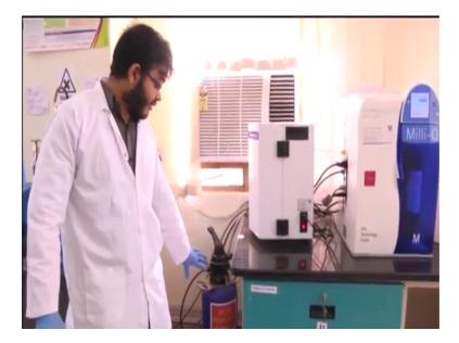
Another very important and basic requirement for molecular biology or biochemical experimental work is the usage of proper quality of water. You cannot just use tap water and carry out different reactions or carry out different experiments, because you do not know what ions or minerals or what the pH of the water in the tap is.
