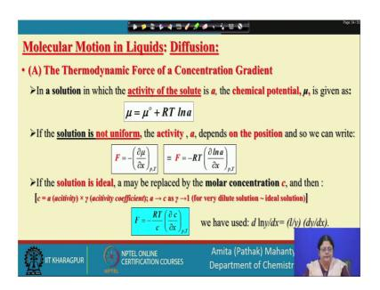
So, this force can how we can relate that force to what we have in a concentrated solution. The thermodynamic force of a concentration gradient see we have talked about the chemical potential in terms of the distance and the slope of chemical potential, we have the gradient in chemical potential we have taken it to be proportional to the force which we have called as thermodynamic force.
