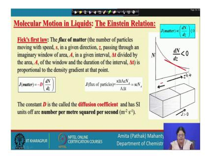
If you remember then if we have a concentration gradient then if I have; if I am moving from or along x axis z axis which is parallel to the container, then how is the flux defined is what we are going to be looking into.
