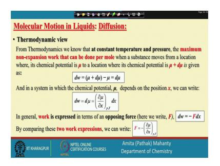
Before that we need to know what is the thermodynamic principle involved. What is the thermodynamic principle involved when you have diffusion or we have a transport through the medium. So, for the most basic of thermodynamics if you remember at constant temperature and pressure, the maximum non expansive work that can be done by a mole of a substance comes from the location, where from the chemical potential from one location to another.
