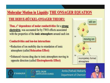
So, what we are trying to explain? We are trying to explain the square root of molar concentration of a strong electrolytes dependence on the molar conductivity and the two effects which is associated with the ionic atmosphere which tends to reduce the motilities of the ion and hence the conductivities other ion interaction reduction of ionic mobility
