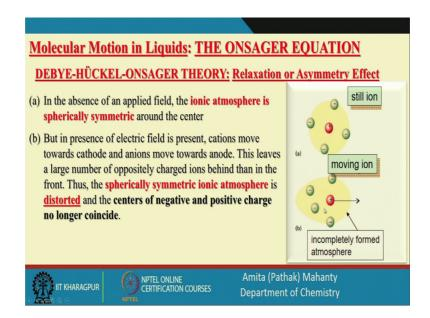
Let us look at this. So, in absence of a electric field what we have the ionic atmosphere is spherical and symmetric around the central ion that is what we have seen, but in presence of a electric field cations move towards the cathode anions move towards the anode we are focusing only on the positive charge; obviously, you will have a negative charge very close by, but we are focusing on one particular central ion to have a simplistic picture ok.
