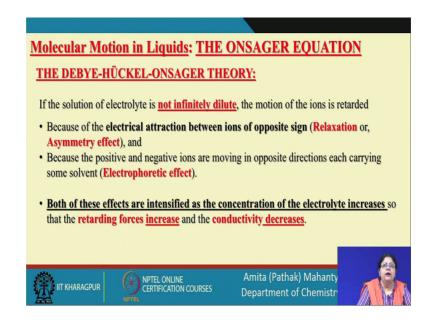
So, when whenever the ions are retarded so, if the ions are retarded in motion; that means, their mobility is reduced both the effects electrophoretic and the relaxation effect it gives rise to a loss in mobility they retard the ion from moving forward and this is hence going to reduce the mobility of each of the ions and hence the conductivity ok.
