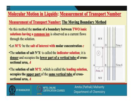
Now, let us first look into the Moving Boundary Method as the name suggests the in this method the motion of the boundary of two ionic solutions have a common ion is observed as the current flows through the solution. So, what we have we have two ionic solutions where one ion is going to be common either the cation or the anion when we are trying to find out the transport number of a cation then we usually take the anion to be as the common ion ok.
