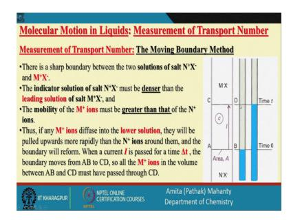
So, there should be a sharp boundary between the two liquids N X plus M X. The indicator solution the indicator solution is this that is N X is denser than the lead solution lead solution is the M X. And one more thing needs to be kept in mind that the mobility of the ion of interest should be greater than that of the indicator of the cation present in the indicator solution ok.
