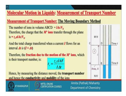
What we have looking into now? We are looking into this zone, this is the zone which we have in which you have what will be the concentration of the number of ions of MA which is going to be present here? The total number of ions which is going to be present here will be the concentration of the ion electrolyte, will be the concentration of the plus ions of the solution into the total number of at would into the Avogadro number.
