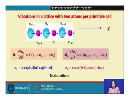
You can have representations of these systems in a more complicated situation where I have a lattice with 2 atoms per primitive cell and here once again, one can write down the equations of motion of the sth plane, but now you have 2 types of planes, one is associated with the blue atom another one is associated with the purple atom.
