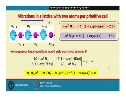
And once again if you solve you find that this is the equation that you need to understand in to need to solve in order to understand what frequencies are possible for the propagation of vibrational waves through a lattices like this.
