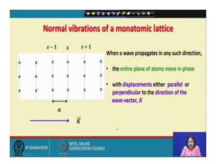
Now, when we talk about these. So, along these directions and along the planes that I have shown in the previous slide, let us say these are the regular arrangement of atoms and if when a wave propagates in any such direction then what will happen this all these planes of atoms will move in phase with displacements either parallel or perpendicular to the direction of the wave vector K.
