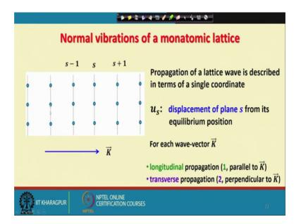
Now, let us try and understand this by taking the actual example of what will happen when this equilibrium picture of a particular direction of propagation this is the direction of propagation of the wave vector K and I have linear arrays of the atoms in this direction arranged in this direction and then what is I am saying is by choosing to represent the situation in this direction, I can describe the propagation of the lattice wave in terms of a single coordinate which is shown here as Us.
