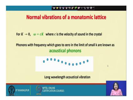
In the limit of small k and these are known as acoustical phonons and this is how they look like and what I am showing to you is the long wavelength acoustical vibration that will correspond to the transverse acoustical, one of the transverse acoustical modes. So, these are representations of the typical normal modes of vibration in a real solid.
