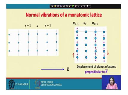
We can also think of displacement of the planes of atom perpendicular to K. So, if you compare these 2 pictures as you see Us remain the same, but this plane has moved in this direction perpendicular to the direction of Kand this plane has moved downward where each atom has moved downward in a direction perpendicular to K.
