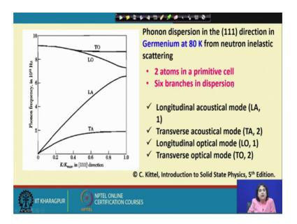
And if you go out and look at the actual experimental data, you will find that for example, as I have shown here for germanium and 80 Kelvin, you can actually find out all the different types of longitudinal acoustic modes, a transverse acoustic modes or longitudinal optical mode or transverse optical mode.
