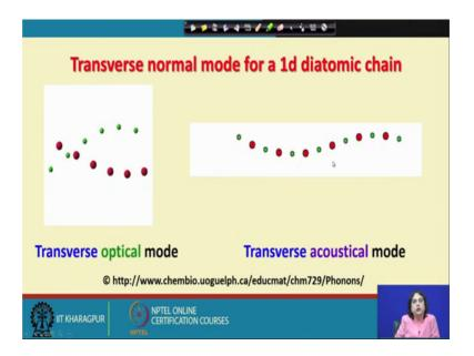
So, these are the typical representations of these normal modes in this kind of 1 dimensional diatomic chain and the take home message over here is that each of these vibrational modes behave as if they are independent simple harmonic oscillators in this given solid.
