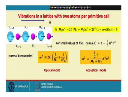
And then you find that there are 2 possible for small values of k, there are 2 possible solutions. For, one set of solutions you have the acoustical modes as before which goes to 0 as k goes to 0, but now you see because of the underlined change in the structure of the solid, you have an additional value of omega and this is known as the optical mode.
