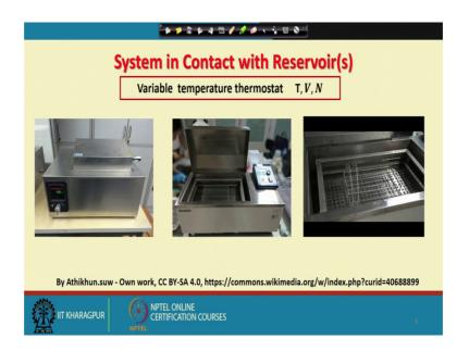
You will see huge chests like this these are the commercially available thermostats. If I open the lid, what you find is there is a compartment inside which can be filled with water and can be heated electrically, and the temperature that you want in that can be controlled from this digital pad.
