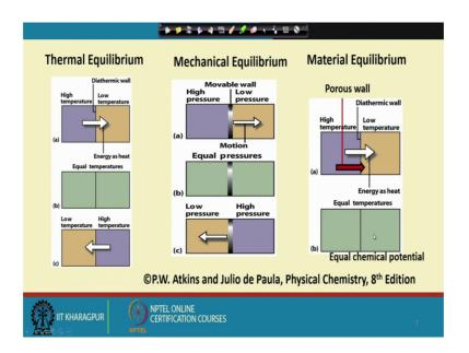
So, this is the case where we have let us say this is the system and this is the surrounding, and the system and the surrounding they are exchanging energy as heat and this wall is a diathermal wall or diathermic wall, and the system will go on exchanging energy with its surrounding till both the parts attained equal temperatures. Under such condition I will say that the system and its surrounding are present in thermal equilibrium with each other.
