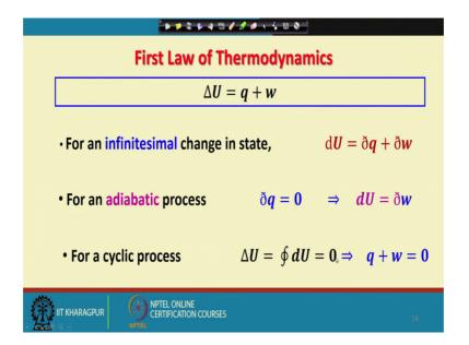
So, for an infinitesimal change dU that is the differential exact differential of the state function U, this is a sum of two in exact differentials this is the infinitesimal amount of heat exchanged between the system and the surrounding. And this is the infinitesimal amount of work done during the change in state.
