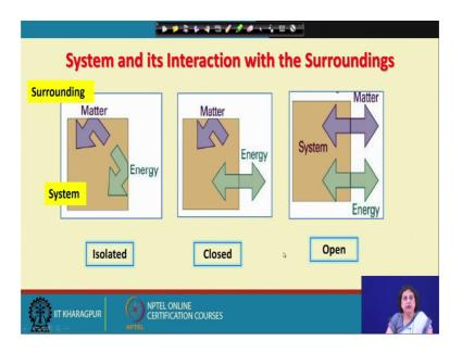
So, here we go. So, first let me point out that this is my system and this white portion is my surrounding. Now the system is surrounded by a wall that is completely insulated as a result of which it cannot exchange energy volume or matter with its surrounding; and we would call such scenario as describing an isolated system. It may so happen that the wall is of such nature, that it allows exchange of energy between the system and the surrounding.
