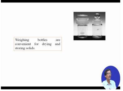
So if you have these weighing bottles and these weighing bottles are very much convenient for drying and storing samples because the entire weighing bottle which is made up of glass like these, these are the 2 examples, the actual examples taken from the school's book again that these are the things and we have to different design. But if you look at minutely, what are the difference between these 2, you have this particular one is the lid is inside this ground glass joint.
