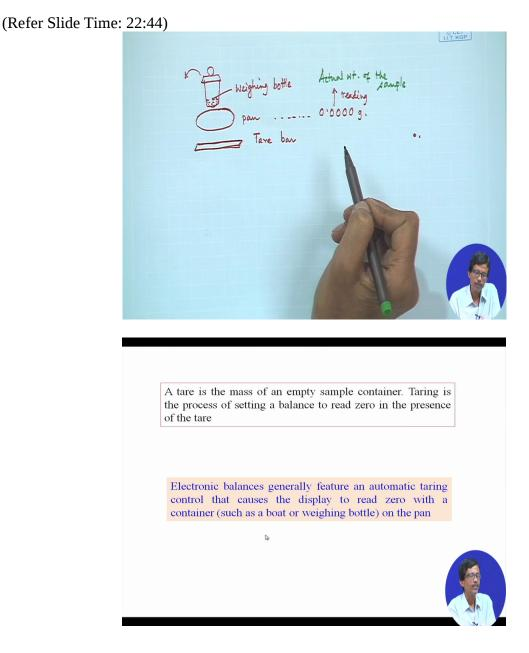
So we can have a look of that particular book. So another particular terminology what we will be seeing over here is how we can use the taring process. So taring of this when we use a weighing bottle for this particular weighing process, so mass of an empty sample container. What is that sample container? How we know that sample container?
