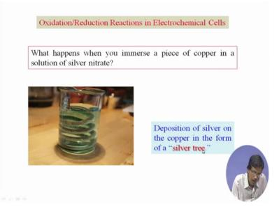
So ultimately these oxidation reduction reactions can give rise to something which we can consider as electrochemical cells, so how we can develop that particular electrochemical cells that we all know from our earlier childhood that a very simple consideration that if we immerse a piece of copper in a solution of silver nitrate, so that means what we are trying to do now as we are bringing copper as the copper electrode and silver nitrate as a solution that means silver ion in the solution.
