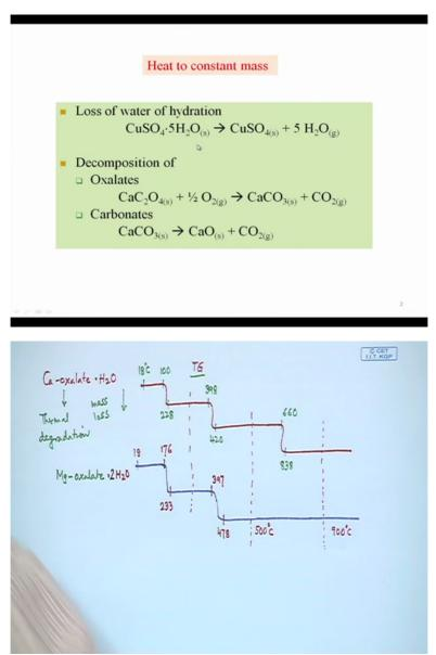
So how do we go for the corresponding thermogravimetric analysis that what we are looking for, we are looking for a heat we are giving to the sample to get some constant mass and this particular constant mass is also an important terminology over here that which particular range you can have a constant mass as it is have a constant mass in this particular range of 18 to 176 when a constant mass within the range of 233 to 397.
