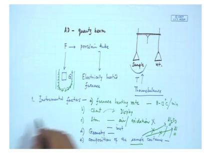
So the beam what we get this A and AD, AD is the beam so we have a AD quartz beam as we all know that a typical balance what is known that is this is can one arm and this is one arm another arm also so what we do we put sample in one arm and the weight on the other so that basic idea we here also will follow to take this and this is the balancing unit. So you have a AD as quartz arm and the interesting thing is that we have a porcelain tube F.
