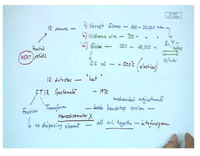
So this give rise to different sources so IR sources so if we heat we all know that heated solids like our body human body which is having at a temperature of 37 degree centigrade we also radiate we also give rise to the IR radiation so the corresponding thermal energy what we release basically that is in the range of IR. So heated solid basically and heated which what particular type of solid it should be INERT, it should not decompose, it should not convert, it
