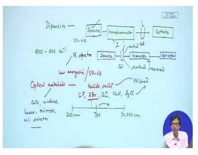
So what we have then all these cases the basic thing that in all cases the instruments what we have the first one is the dispersive one where like that of our invisible spectroscopy we have the corresponding source and we get this particular source through monochromator and we all know that this particular one where we get this monochromator and then finally we go for the detection.
