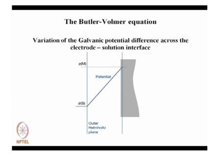
Next, we will concentrate on Butler-Volmer equation, this is another equation. So, variation of galvanic potential difference across the electrode and solution interface. So, this is your metal, this is your solution, phi M, phi S. This is your outer Helmholtz plane. So, this is the potential function, as a function of distance. So, this is phi M, this is phi S and with distance it follows some curve.
