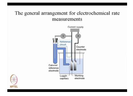
This is the general arrangement for measurement of electrochemical rates, as I told you earlier, that it is basically do a current potential diagram. It is a arrangement for doing a current potential diagram, so basically, if you think of your Tafel plot or may be the Butler-Volmer plot, everywhere you see that it is you are plotting your current density. Current density means it is basically difference of your anodic and cathodic.
