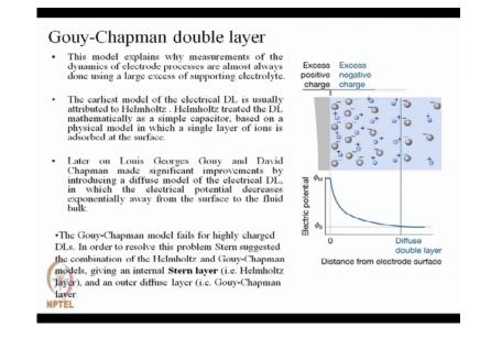
Gouy-Chapman double layer model is another model. This model explains why measurements of the dynamics of electrode process are almost, always done using large
