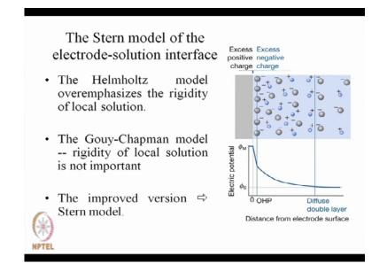
Stern model of electrode solution interface, you see here very close up to outer Helmholtz plane, it is behaving like Helmholtz double layer, and beyond that it is Gouy-Chapman. The Helmholtz model overemphasizes the rigidity of the local solution. The Gouy-Chapman model, for the Gouy Chapman model, the rigidity is not that important and improved version is your Stern model, as I talked about. So, here it is decreasing almost linearly and then exponentially up to the diffused layer.
