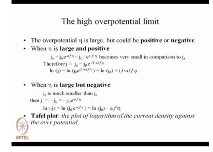
Next is, what is going to happen when we are in the high over potential limit that is eta is large, greater than or equal to 0.12. Then, it could be, I mean over potential large, means it could be large in positive sense or large in negative sense also. If it is large positive what is going to happen? Then that cathodic current density j c is equal to j 0 into exponential minus a f eta and which becomes very small in comparison to j a.
