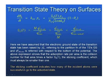
So, so what do we get we get d theta A d t that is rate of reaction which is equal to k T S T into P A and you write the respective expression for k T S T from the previous slide that S 0 T P A S 0 T P A S divided by N 0 twice pi m k B T into 1 minus theta A where S T is given this expression q double dagger 2 D vibration divided by q translation of the unit cell in two dimension because unit cell means it is a two dimensional case therefore,
