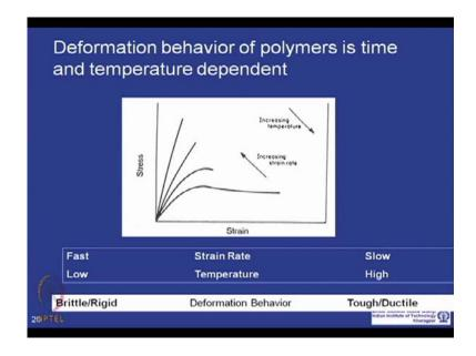
So, just again showing the same thing, with increasing temperature, the sample become stuff and ductile. With reducing temperature, becomes brittle and rigid whereas, applying high strain rate, makes the sample brittle and rigid, very slow strain rate mix the sample tough and ductile.
