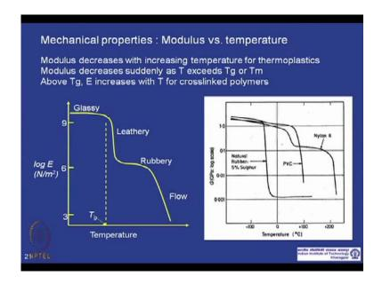
The modulus which means, the stiffness or rigidity, very much depends on the temperature, as I said so, this is the example, how the modules changes with temperature. As we know that, the polymers have undergo glass transition and melting transition at at a adiabatic temperature for example, if you pure amorphous material undergo go glass transition T g whereas, semi crystallized polymers undergo both glass transition and a melting at T g and T m subsequently.
