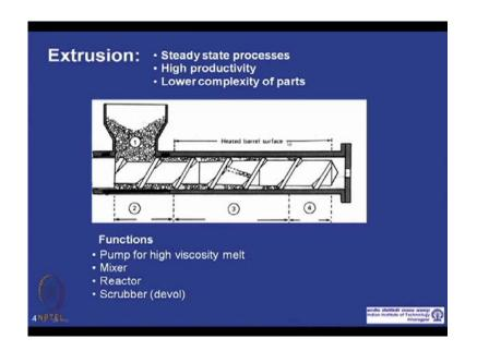
Talk about briefly extrusion process, extrusion process as said, this is steady step process, this is continuous process having high productivity and it is used for making low complexity of parts like pipes sheets and so on. This is a schematic or structure or a scheme of a extruder where extrusion is made, a one screw is shown, this is a single screw extruder. That in some other cases, there could be two screw, which makes that instrument as twin screw extruder.
