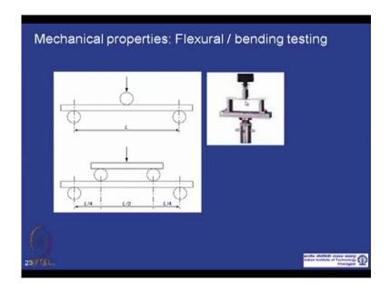
This is another mechanical property testing, we just discuss all last few minutes about tensile basically, the stresses is applied in a longitudinal direction. Here, in case of flexible or bending testing is basically bending mode where, the stress applied. It could be three point bending test or four point bending test, is like stresses or strain is applied in bending direction so, higher the modulus as bending will be lower.
