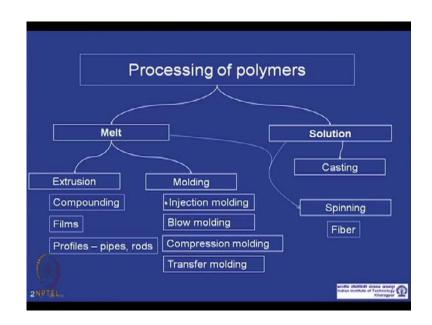
So, let us start our discussion on polymer processing very briefly as I said, polymer processing can be done from a melt state or a solution state. Melt state, there are two three techniques mainly, extrusion, molding, thermoforming, by which the polymer converted to final specimen. And for solutions, we can do casting is applied to making films and spinning is applied to both from polymer melts or polymer solutions for example, making fibers.
