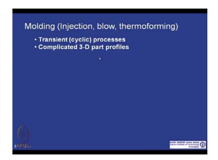
So, going to molding and molding is a cyclic transient process and is molding can be used for making complicated three dimensional parts, as I said it could be injection molding, blow molding, thermo forming.
