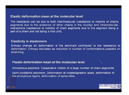
What happen to in at the molecular level, in inelastic during elastic registration, the the resistance to deform the resistance to deformation can happen both intermolecular. The polymer chains are you know entangle to each other so, polymers, the resistance to deform may happen, because of presence of the other polymer chain segment in the near
