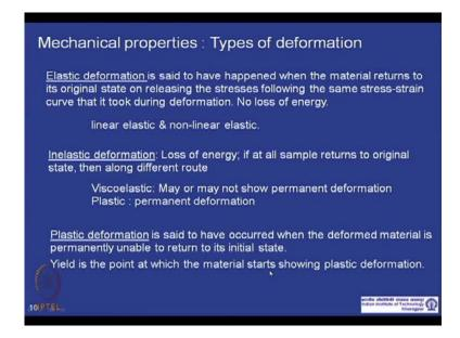
Now, mechanical probabilities is polymers, mechanical prosperities is related to deformation, what happened in when you apply some force or a stress to polymeric material or plastic material, it it deforms. And the deformation (( )) is basically a but, what we discussed, what we talked about mechanical properties. So, you first know, how many different types of deformation that a polymer undergo, under applied stress or applied force.
