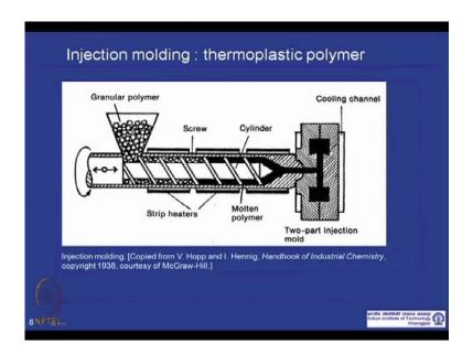
Injection molding is done mainly for thermo plastic material and it is similar to the extruder machine, there is a hopper where, you add the gremial polymer material and some additives, which act as a mold release agent. So that, after the part is formed, it can easily taken out from the mold, there is screws, it basically melts and mix those those polymers with additives here and this screw by rotating it, takes it forward.
