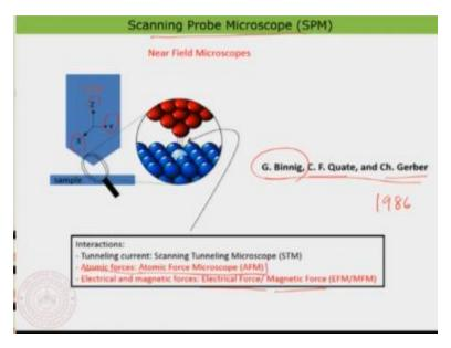
So, it again comes under the bigger family of scanning probe microscopy. So, that something we have already talked about and you were also seeing this. So, in this case also what we have here again here is a probe which is actually able to move along the x z and y direction. So, that is quite important. So, you can basically just move them like this and you can retract them, approach them. So, you can basically just do a three dimensional scanning using this tip.
