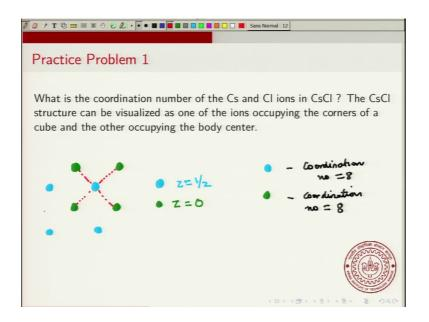
So, I will do a few problems fairly straight forward problems. So, the first problem is asked you what is the coordination number of cesium and chloride ions in CsCl? And it is said that the CsCl structure can be visualized as one of the ions occupying the corners of a cube and the other occupying the body center.
