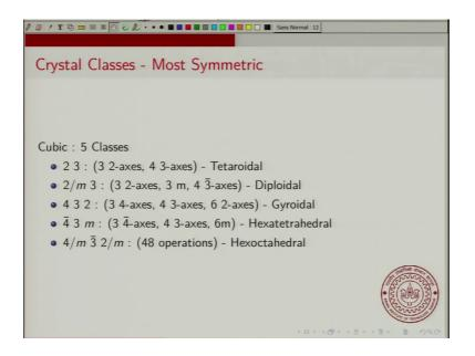
But the most the highest symmetry; the crystal class with the highest symmetry the crystal system with the highest symmetry is the cubic system. And the cubic system is gives the most symmetric classes. There are five crystal classes in the cubic systems, and these have names, ok.
