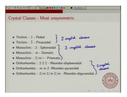
So, let us first look at the most un symmetric crystals ok. So, if you look at the triclinic system that has the least symmetry. So, actually there is no essential requirement of symmetry ok. So, if there is only, if the only symmetry operation that is present is an identity; identity which is basically mean means doing nothing.
