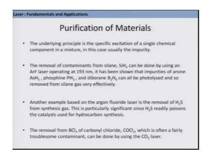
Also we can use this you know laser radiation for purification material and here the underlying principle is the specific excitation of a single chemical component in a mixture, in this case usually the impurity.
