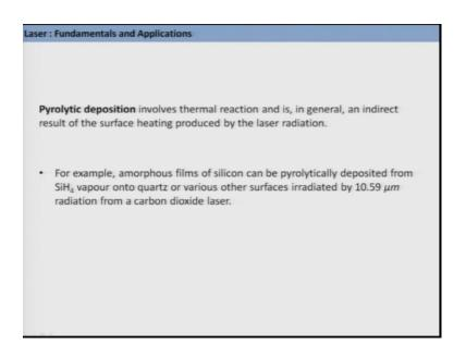
Now individually if you look at pyrolytic and photolytic decomposition the photolytic decomposition involves thermal reaction and is general and indirect result of the surface heating produced by the laser radiation.
