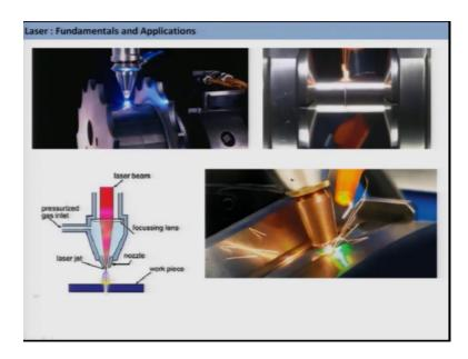
So, here like you know two parts are being you know joined together well together by using the laser same is done on the right side image and this is a schematic of the process where the laser beam is focused using a lens and you know this is passed through nozzle where through also you send in you know some gas under high pressure. So, that you know you can create the exact environment on the metal surface which you are trying to weld is created.
