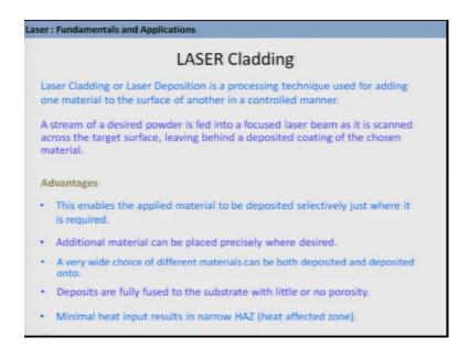
So, the laser cladding or laser deposition is a processing technique that you know is used for adding one material to the surface of another in a controlled manner and for this a stream of desired powder is fed on to into a focused laser beam as it is scanned across the target surface, leaving behind deposited coating of the chosen material.
