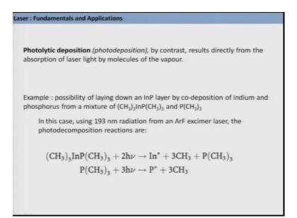
On the other hand photocatalytic deposit sorry photocatalytic deposition result directly from the absorption of laser light by the molecules of the vapour. So, here we provide another example where this example is you know materialized by using 193 nanometer laser light from excimer laser.
