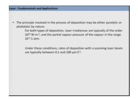
And the principle involved in the process of deposition in this manner can be either pyrolytic or photolytic by nature. Now both the types either by pyrolytic or photolytics of this deposition the laser irradiance is a typical in the range of 10 power 12 watt per centimetre square and the vapour pressure of the gas is required to be between you know in atmosphere to 1 milli bar ok.
