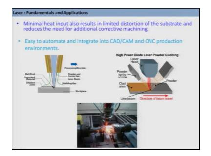
And this, because of this you know narrow region of the focal spot which in turn in case the minimal heat input that results in limited distortion of the substrate and reduces the need of additional collective machining, certainly a big advantage.
