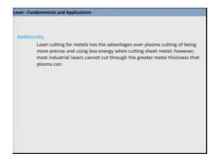
One additional thing I would like to mention here is that the laser cutting for metals has the advantage over plasma cutting of you know because it can be more precise and using less energy when cutting sheet of metal.
