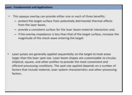
Now this opaque overlay can provide either one or each of the following benefits. For example it I can protect the target surface from potentially detrimental thermal effects which is; obviously, you can you can expect from laser beam. Second it can provide a consistent surface for the laser beam material interaction and third if the overlay impedance is less than that of the target surface increase in the magnitude of shock wave entering the target.
