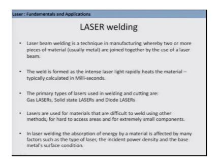
So, let us start by talking about laser welding. So, a laser beam welding is a technique in manufacturing where by two or more pieces of material easily they are metals are joined together by the use of a laser beam. So, conventionally what is done you know when you want to join two metals then you come with a very high temperature flame and then you know join them together that is known as conventional welding.
