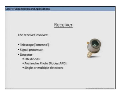
On the hand you have to receive on the n th and the receiver can be some detector like you know it can be, it can be like an antenna, with a telescope system having a detector like you know PIN diode or avalanche photodiode or you know like you know and you know pmt basic detector or cc based detector they all can act as a receiver of the signal.
