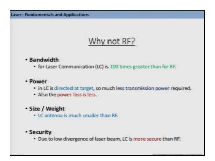
And if I again ask them fine I understood about the fiber optic network why not then why not radio frequency. So, here is the problem is a bandwidth for laser communication the bandwidth is 100 times better than that for radio frequency in terms of power in laser communication system is you know laser communication system is directed at target. So, so much less transmission power is required and more over because it is a direct communication the loss is also very less.
