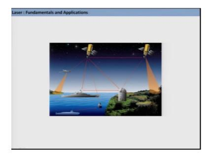
So what are the security aspects? Free space laser communication systems have narrow optical beam which are not accessible unless viewing directly onto the transmission, but as what I was saying, so less divergence. So, you know very less chance of interception of that particular information that is being passed.
