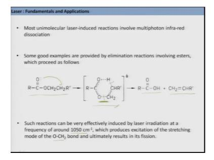
Now most unimolecular laser induced reactions involved multiphoton infrared dissociation. Let us get some good examples, so one good example is the elimination reaction involving esters which process as shown in this scheme. So, you have an ester, so it is like C double bond O and O R, are is an alkyl group, and this is the transition state.
