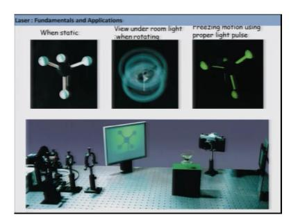
What should be the resolution of your light flash? So, that you can take the image at a as if the molecular model is stationary, so this is the image of the stationary model and when you allow it to rotate it appears like this this is a real image of a rotating model. So, you can immediately figure out that this is totally fuzzy right you cannot figure out whether there is a molecular model or there is you know something else.
