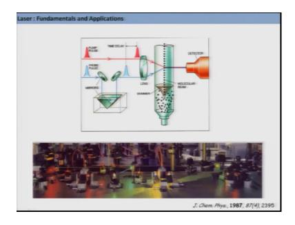
So, one needs to do a proper arrangement of doing the experiment as was done by Ahmed Zewail, where you have one pulse which excites the molecule and in the second pulse probe that excited state. So, essentially if you are you know trying to figure out what happens between this CH3 I and sodium. So, how the transition state, so you create that you know molecule in the excited state, so the transition state is created and then how it evolves with the time you come with a second pulse.
