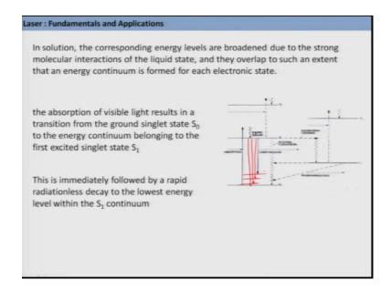
So, earlier we mentioned that like solid state lasers, this dye laser also gives much broader fluorescence spectrum and that is you know good in many senses and this broadening takes place due to the interaction of this molecules with the surrounding environment and because they are you know freely moving around.
