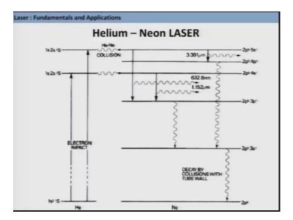
So, here I show you the energy state diagram for this helium neon system; so, you can see the energy states of helium and neon they are very much comparable and this is very much beneficial. So, what is done first the electron discharge will provide the electron impact so the electron impact will cause the excitation from helium; 1 s state to helium 2 s state; so, and also to this sorry helium 3 s state and also to 1 s state.
