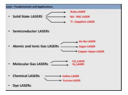
And we can categorize them into different sections like solid state laser, semiconductor lasers, gas lasers atomic as well as molecular gas lasers, chemical lasers dye lasers and so on so forth. So, today we are going to look into different types of laser belong into this different categories. So, we will start with the solid state laser. And the first one that we will look at is the ruby laser.
