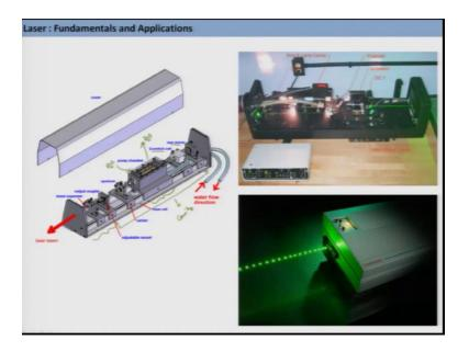
So now I will show you how an Nd YAG laser is constructed, how it looks like you know actually. So, this is the region. So, this part is the heart of the system, where you have the Nd YAG crystal and the flashlight flush lamp that kept. So, here also the same technique is used that is you wrap this flash lamp and the Nd YAG crystal in a elliptical reflector tube. Now there are some practical concerns, this flush lamp is you know flushing and it keeps very high amount of photon intensity.
