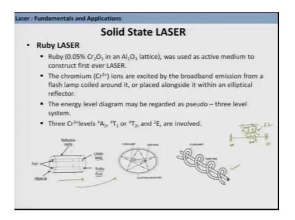
So, this was about the energy level diagram of this system. Now as I was saying how experimentally it is done. So, this ruby crystals they are like you know like innovative rod. So, if you place this ruby rod and this lamp which is like a you know tube linear tube side by side, then you can you know this lamp can excite this ruby crystal.
