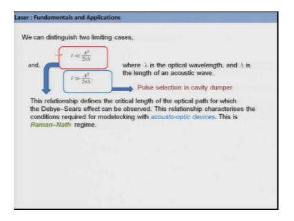
And then two limiting cases essentially; one is this one, where the optical path length is you know far less than the quantity given by capital lambda square by 2 pi lambda and the other limiting case can be the optical path length is much much much greater than capital lambda square by 2 pi lambda. We are not bothered about how did we come to this conclusion because that is not a part of this particular course curriculum, but we will just look at these two you know values that can be obtained.
