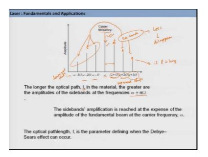
So, the central part this omega is my incident frequency and this frequency is being modulated by this amount, this amount or in this side. So, this is the you know upward shift and this are the downward shift; so this guys. So, these are called side bands because they were not there earlier. So, this is my main band that is also known as the carrier frequency and these side bands are created.
