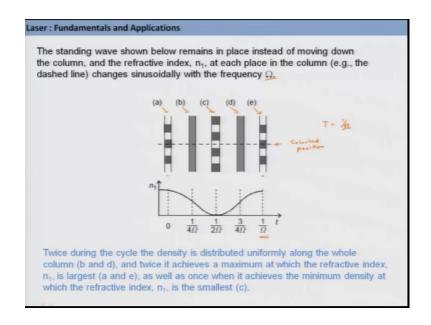
So, here we have given five different situation for the same type of column through which acoustic wave is being sent and essentially that is forming the acoustic standing wave. So, we have given situations a to e; you can see that you know there are different modes are possible. And a to e essentially covers from time 0 to the full period time which is given by 1 upon omega.
