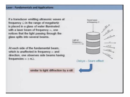
So, we said that this effect is known as Debye Sears effect and this Debye Sears effect is analogous to a diffraction except for the fact that in case of like diffraction you know by a slit does not change the frequency of light, it just modulus the intensities.
