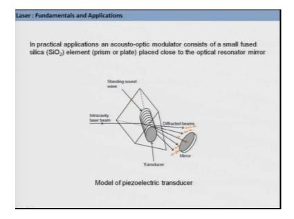
Now, how do you do that practically? So, you need to use an acousto optic modulator. So, this acousto optic modulator generally can be as I said in one of the previous classes it can be like fused silica and this is one of the most used systems. So, if you take small prism of fused silica or small window of fused silica and place it extremely close to the optical resonator mirror then, what will happen that is shown in this picture given here.
