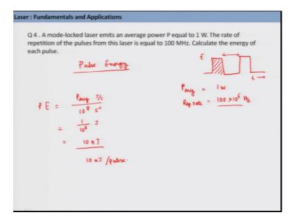
Now the next question also it talks about a mode lock laser. So, you can you can ignore this mode lock thing here. So, now, the question is that if the this laser emits an average power P which is equal to 1 what the rate of repetition of the pulses from this laser is equals to 100 megahertz calculate the energy of each pulse. So, essentially this question asks about pulse energy.
