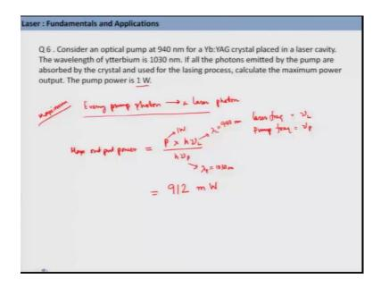
So, let us look at this next question. So, consider an optical pump act 940 nanometer for ytterbium YAG crystal placed in a laser cavity the wave length of ytterbium is 1030 nanometer which means that you know when it fluoresce the stimulated fluorescence has a wavelength of 1030 nanometer. If all the photons emitted by pump are absorbed by the crystal and used for lazing processes calculate the maximum power of the output and the pump power is given right 1.
