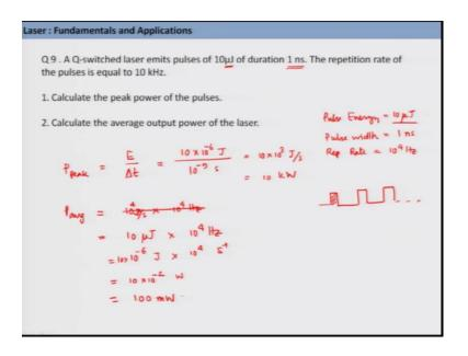
So, here last question that we will look at is if we take a Q-switched laser that emits pulses of 10 micro Joule of duration 1 nanosecond and the repetition rate of the pulses is equal to 10 kilohertz. So, what I have we have pulse energy you see you have to notice the unit rate, so this is 10 micro Joule. So, it is pulse energy that is equals to 10 micro Joule and pulse with the duration is this.
