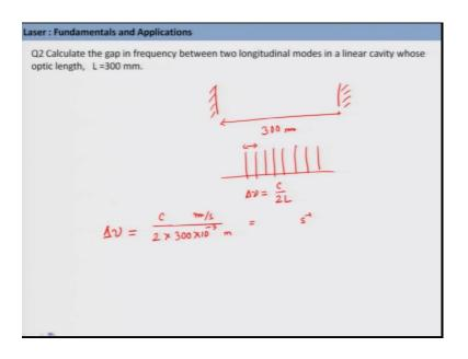
So, we are supposed to calculate the gap in frequency between two longitudinal modes in a linear cavity whose optic length optical length is 300 millimeter. So, essentially you have a cavity and it says linear cavity. So, that is what we have discussed we did not discuss any other type of cavities that are possible. So, essentially this distance is 300 millimeter.
