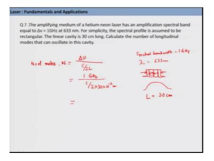
So, the question next question is the amplifying medium of a helium neon laser has an amplification spectral band equal to delta nu because to 1 gigahertz.
