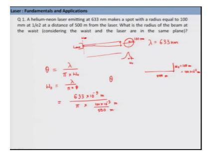
So, the problem states a helium neon laser emitting at 633 nanometer makes a spot with a radius equal to 100 millimeter at 1 upon e square at a distance of 500 meter from the laser.
