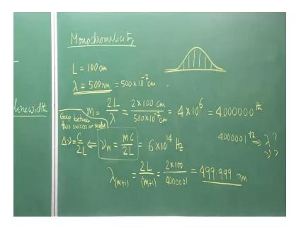
So, if I take a cavity length 1 100 centimeter, and the wavelength output of the laser of that particular one particular mode as 500 nanometer which is in centimeter unit I have this value. So now if this is my output then can I find out which mode it is. So, what is the value of m that we used earlier right. So, if I have to find m then what is the value it is because m lambda equals to 2 l that we have seen just few minutes back.
