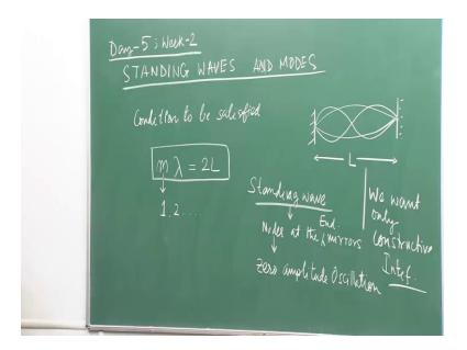
So, what are these? So, we created this cavity right. So, you have the active medium here. So, you are pumping and then your light is you know going and bouncing of between these 2 the length of this cavity is I lambda is the wavelength of the light. So, if I can you know have the information regarding lambda I can very easily get the information for frequency because they are related by the by the speed of light ok.
