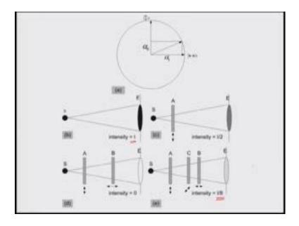
So, the source whenever it was directly measured it was of some value and then as it was put through these different changes we were able to see how these things are getting broken up. So, if the split at each place is half then we expect at every point of a beam splitter measure at the end an intensity which would be in the order of one-eighth of the original intensity which is measured because at every element only 50 percent of the light is going to come through.
