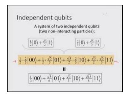
So, these are Independent qubits so that they could come together and we can have a system of 2 Independent qubits which are 2 Non Interacting particles for examples as we take here each having zeros and 1 qubits and when we put them together then we land up producing these total combine system which will be eventually looking at the kind of
