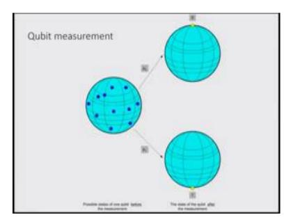
So, the qubit measurement; however, will give rise to the two probable conditions one with probability p 1 of finding it in 1 and probability of p 0 finding it in 0, but all possibilities before the measurement exists.
