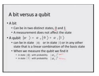
So, that is why a bit can be in two distinct states only 0 and 1 and the measurement of one does not affect the other; however, for a qubit it is going to be in the superposition of both of these conditions can be in state 0 or in 1 or any other state that is a linear combination of the basis states; when we measure we find it has a probability of finding it in state 0 with probability of the coefficient square of each of these states depending on which we measure.
