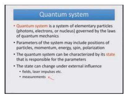
Now, Quantum systems that we have been using are the ones which are of elementary particles nature. So, for example, photons, electrons and nuclei that is governed by the laws of quantum mechanics.
