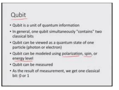
The qubit is the unit of quantum information for us in quantum computing and in general 1 qubit can simultaneously contain 2 classical bits.
