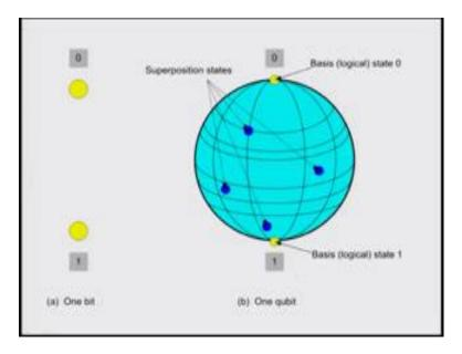
So, in some sense a single qubits will be possible; will have all the possible superposition states in addition to the basis logical states of 0 and 1 whereas, the bit can only have two possibilities 0 and 1.
