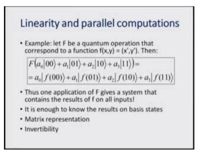
And the principle of parallel computations which is followed in quantum computing; so, if we have F as a quantum operation that correspond to a function f of x taking to x prime to y prime; then the quantum operation has to be such there it will be doing a linear processing of the entire system and one application of F gives rise to a system that contains the result of f in all the inputs.
