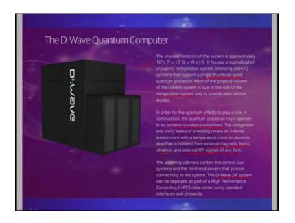
So, that is the basic idea behind this in terms of the actual computer it sort of looks like this where the physical foot print of the system is about 10 feet by 7 feet by 10 feet in terms of it is length width and height, it houses a sophisticated cryogenic refrigeration system because we are talking about very low temperatures, shielding an input output systems that support a single thumbnail sized quantum processor.
