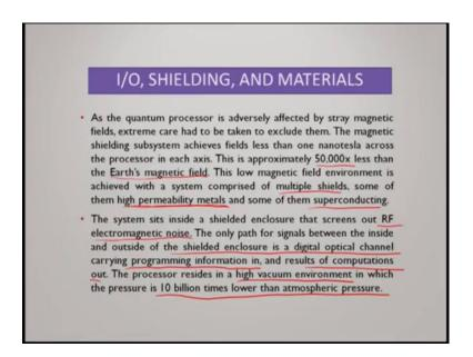
As the quantum processor is adversely affected by stray magnetic fields extreme care had to be taken to exclude them. The magnetic shielding subsystem achieves fields less than 1 tesla across the processor in each axis, this is the approximately 50000 times less than the earth magnetic field, this low magnetic field environment is achieved with a system comprised of multiple shields, some of them high permeability metals and some of them superconducting.
