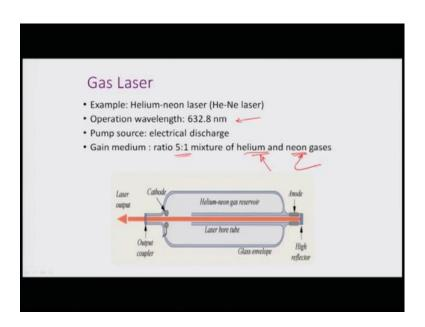
The gas laser typically once that they use now days are in the visible region of 632.8 nanometers, so electric discharge, and the gain medium is the ratio of 5 is to 1 mixture of helium and neon gases. The helium is been excited and been passed on to the neon gas energy process goes inter conversion into the neon gas which is the one which is our active place medium in this particular case.
