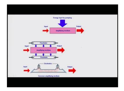
Roughly speaking we have the electrodes and where the gas amplified mixtures are put. If we want to look at as high voltage which is creating the discharge, and that is what is shown here amplifying medium the flash tube is doing that and we get the laser tube.
