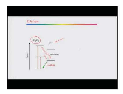
So, we already know of the chromium active ion which is essential for the ruby laser for instance. The host is the alumina which is the reason of the ruby crystal it acts as a host, whereas the chromium is the active medium which leads to the lasing for the system.
