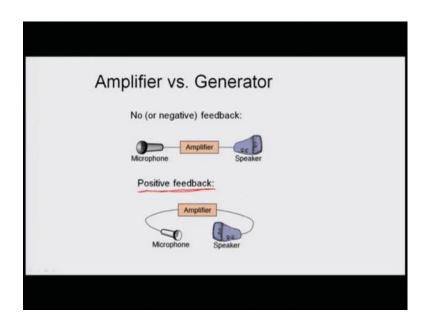
So, this is the principle that we use here in which we more have the idea with positive feedback where the amplifier is being fed back into it and its cartoon wise it is like you know here is the picture we have the microphone face in the speaker and then it will be a lot of difficulty in this process where we know that here a high screech, because the microphone is feeding into the system and you have lot more amplification that you need.
