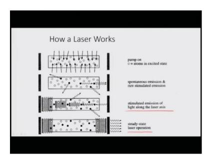
So, crudely speaking this is how a laser works. We have a the laser beam is pumped, atoms in the excited state has been generated, spontaneous emission and rare stimulated emission is happening, and that is being put inside and because stimulated emission is something which is along one direction and is directional so what happens along direction of the cavity its gets amplified.
