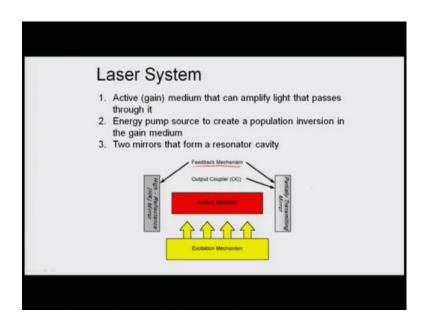
In some sense the laser system can be lead once again we looked at as the active medium which is being excited or being pumped by the excitation mechanism, and which is being put inside a resonator one of the sight to have the feedback mechanism. The part, from which some part of the energy being taken out, technically is known as the output coupler. And the other sight from which almost no light or the no energy indication is happen is known as the high reflector.
