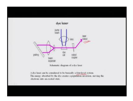
Typically, in this process there either a dye cell or a dye jet into which the pump is being focused and that sets of the cavity where there can be different ways of selecting the wave length by using a grating or prism, and then there is this cavity which is inside which the laser is been put so that you can get the output.
