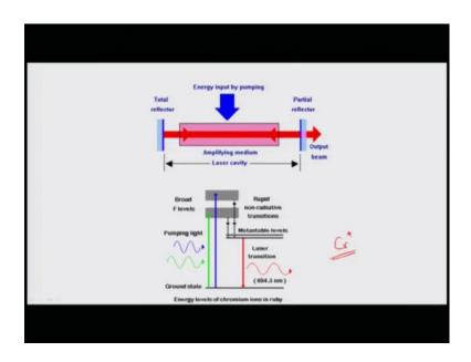
This is the basic principle; he used a electrical pumping by using the electrode to pump the laser system from the lasing medium, which is the ruby in the particular case. And that is how he got it the energy input was laterally provided which was the amplify medium and this is what the chromium ions; those where the once which are necessary in the ruby crystal which gave rise to the lasing material.
