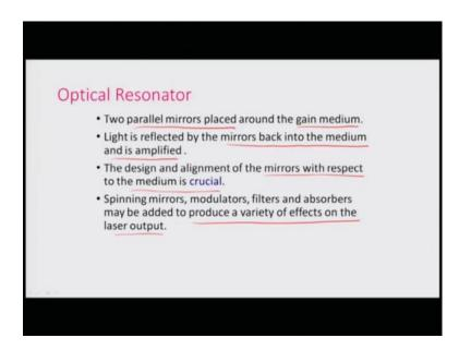
The resonator is the two parallel mirrors placed around the gain medium. The light is reflected by the mirrors back and forth into the medium and is amplified. The design and
