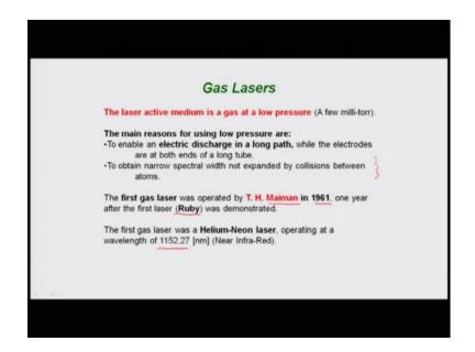
The pump source is a flash lamp in this case and then the ends of the ruby rod serve as laser mirrors the basic idea of this. Again for gas lasers where the example a laser active medium is the gas at low pressure roughly a few milli-torr, the main reason for using the low pressures are to enable an electric discharge.
