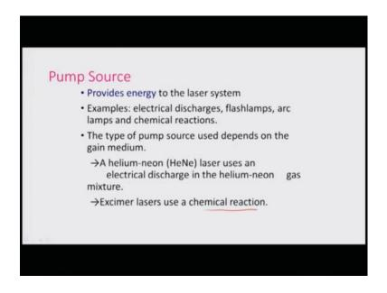
The pump source provides energy to the laser system. Examples include electrical discharges, flash lamps, arc lamps and chemical reaction as we mentioned. The type of the pump source depends on the gain medium. For example, helium-neon laser uses an electric discharge in the helium-neon gas mixture; excimer lasers use a chemical reaction and so on and so forth.
