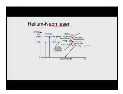
And one of the lasers in this category is helium-neon laser where the helium and neon are put together inside the system, inside a gas cell. And the helium is excited which then transverse the energy by collisions to neon which as those exact met stable energy states where from the lasing can occur and to its higher excites states which are not the ground state. And therefore, lasing is much easier because a 4 level system.
