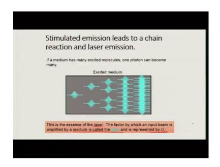
So, it can look something like that. The stimulated emission leads to a chain reaction and laser emission. So, this is the cartoon of such a situation; if a medium has many excited molecules one photon can become many and here is a cartoon showing that in availability of inverted system would allow for multiple photons to be generated from itself so much so that you finally get an output and this is the essence of the laser.
