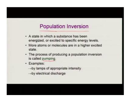
So, in order to look at into something known as this very important term of population inversion; a state in which a substance has been energized or excited to a specific energy levels. More atoms or molecules are in a higher excited state than in the ground state. The process of producing a population inversion is called Pumping; these are all the details that we have done. The examples of such process can be by the use of lamps of appropriate intensity or by using electrical discharge.
