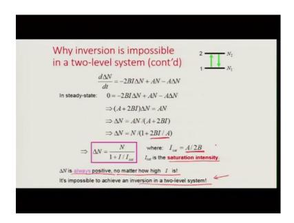
And at study state what will happen is the rate of change would be equal to 0; because whatever goes to the excited and ground ability becoming 0. So, in that case we get a situation where the we have the change that we are looking for delta N; it is going to be total numbers over 1 plus I over I of saturation.
