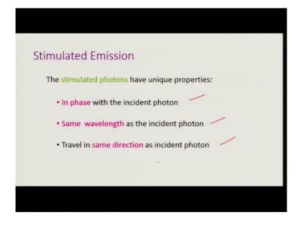
So, the stimulated photons have unique properties which are in phase with the incident photon, same wavelength as the incident photon and travel in the same direction as the incident photon; essentially giving rise to the principle of the laser.
