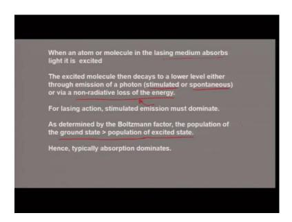
When an atom or molecule in the lasing medium absorbs light it is excited. So, that is the absorbing process. The excited molecule then decays to a lower level either through emission of a photon which can be either stimulated or spontaneous or via a non radiative loss of the energy. Now in this particular case of non radiative loss of energy this is not doing anything to us is just a loss factor.
