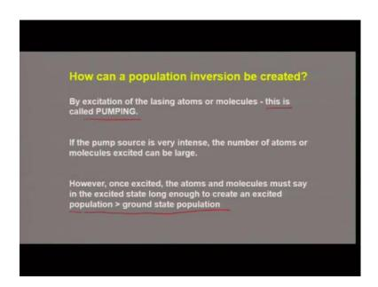
So, we can ask the question how a population inversion can be created. One way of looking at it is by exciting the laser atoms or molecules and this process is called Pumping. If the pumps source is very intense; the number of atoms or molecules excited can be large. However, once excited the atoms and molecules must stay in the excited state long enough to create an excited population which is greater than the ground state population.
