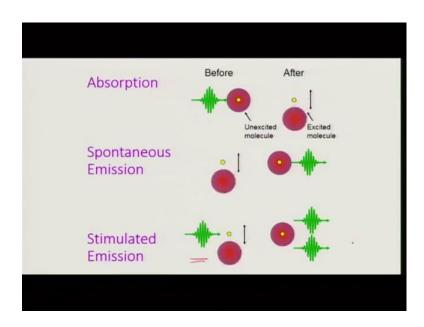
Pictorially this is what we are looking at; we have unexcited molecule which is being excited by the radiation; we get the excited molecule if it under goes just simple emission of photon then it is spontaneous emission; however, if you another photon available for it to bring it down to the ground state then we get stimulated emission which is the one with the phase.
