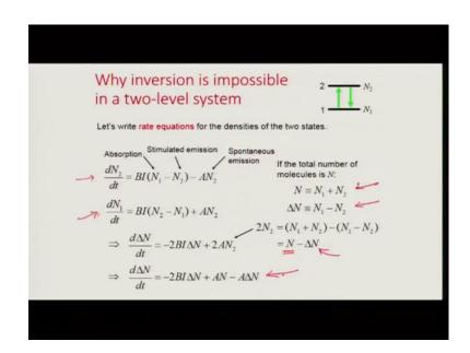
So, the first question to ask them is that what happens when we consider the simple case that we have been treating right now; the two-level system. It turns out that inversion is actually impossible in a two-level system. So, how do you look at it? So, here is the going back to the rate equations; we can write how the population would change with respect to time based on these expressions that we have just devised.
