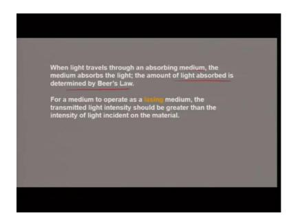
When light travels through an absorbing medium the medium absorbs the light; the amount of light absorbed is determined by Beer's Law which we know; which means that the moment we have photon being absorbs the light availability as it goes through the system keeps on going down. So, for a medium to operate as lasing medium the transmitted light intensity should be greater than the intensity of the light incident on the material.
