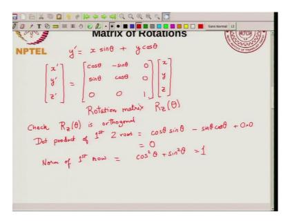
What else can you do? You can also write the y prime. So, I can also write y prime is equal to and by the same method what I will get is y prime equal to x sin theta plus y cos theta. So, our three transformations are basically z prime equal to z, x prime equal to x cos theta minus y sin theta and y prime equal to x sin theta plus y cos theta.
