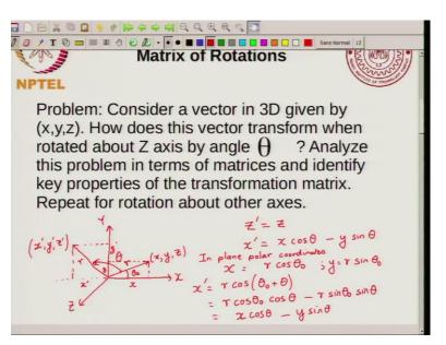
So, the problem is tough, I will just state the problem in the following way. So, suppose you consider a vector in 3 D and let us say that vector is given by x, y, z. How does this vector transform when it is rotated about Z axis by angle theta? And what I said is analyze this problem in terms of matrices and identify key properties of the transformation matrix and repeat for rotation about other axis.
