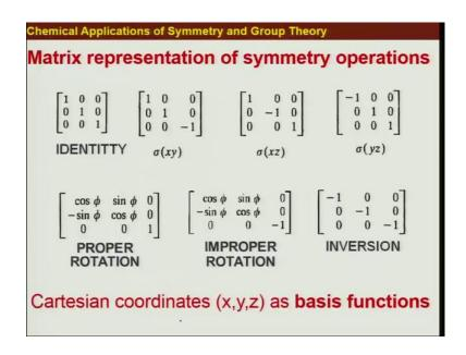
And on your screen you can see all the matrix representations that we form for different symmetry operations. For example, identity difference sigma planes, proper rotation and improper rotation as well as inversion symmetry operations. In order to form this representations we choose x, y and z coordinates of the Cartesian coordinate system. So, x, y, z acted as a basic set for forming these representations. So, you can look at all these representations that we formed in the last class.
