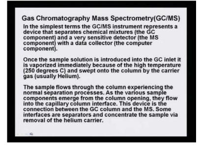
In the simplest term, the G C M S instrument represents a device that separates chemical mixtures; that is through the G C component and a very sensitive detector that is the mass component with a data collector which is the computer component. So, basically it is made up of 3 components.
