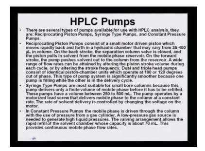
HPLC mobile phase are controlled by pumps. There are several types of pumps available for use with HPLC analysis. They are: reciprocating piston pumps, syringe type pumps and constant pressure pumps.
