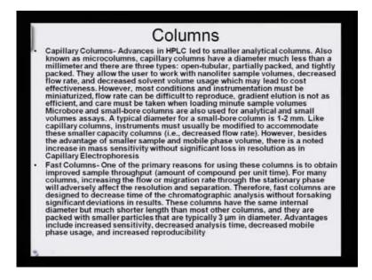
Columns are of the capillary type, which are also being used, because everywhere micro analysis is becoming very, very important. So, just like we have capillary columns in GC, we also have capillary columns for doing smaller analysis or micro analysis using capillary columns.
