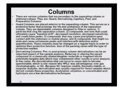
Columns - there are various columns that are secondary to the separating column or stationary column. They are called: guard column, derivatizing column, capillary column, fast and preparatory column. Now these are varieties of columns, which are used at different instances.
