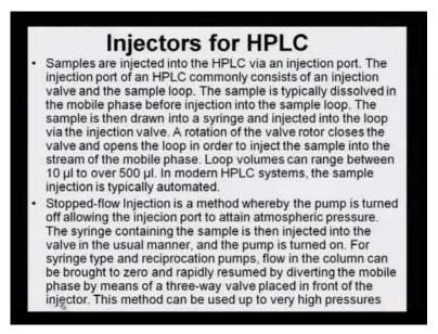
What are the different types of injectors in an HPLC machine? As what we had a different set of injectors or injection mode for GC, similarly, there are options of injectors in HPLC too.
