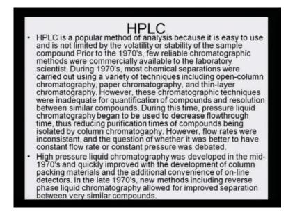
HPLC is the abbreviation for it. HPLC is a popular method of analysis, because it is easy to use and is not limited by the volatility or stability of the sample compound. Prior to the year 1970, few reliable chromatographic methods were commercially available to the laboratory scientist. During 1970s, most chemical separations were carried out using a variety of techniques including open-column chromatography, paper chromatography, thin-layer chromatography.
