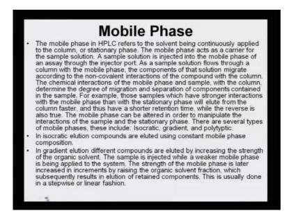
The mobile phase in the HPLC refers to the solvent being continuously applied to the column or stationary phase. The mobile phase acts as a carrier for the sample solution; that is what helps the sample to move further.
