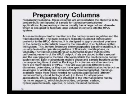
Preparatory columns are of course for bulk separation. These columns are utilized when the objective is to prepare bulk or milligrams of the sample for the laboratory purpose application. The ideal example for preparative column usage is in pharmaceuticals; you know, when the intermediate compounds have to be separated, and further on more reaction have to be done, it has to be done on a little larger scale. So, columns could be analytical type or they could be preparative type.
