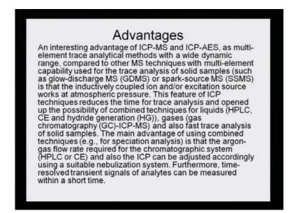
Advantages - an interesting advantage of ICP-MS and ICP-AES, as multi-element trace analytical method with a wide dynamic range compared to other MS techniques with multi-element capabilities used for the trace analysis of solid samples such as glow discharge MS, that is GDMS or spark-source MS (SSMS) is that the inductively coupled ion and/or excitation source works at atmospheric pressure. So, these work at a very ambient atmospheric pressure.
