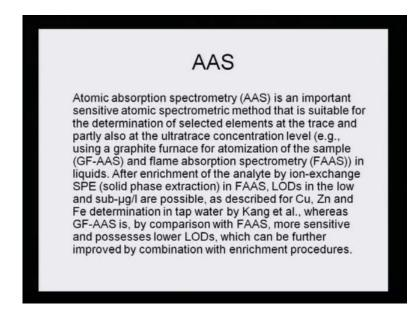
AAS of course, you have seen that the flame AAS is not very sensitive method. However, it is sensitive enough to analyze that is suited for the determination of selected elements at trace and partly also, at the ultra-trace concentration, if we are using graphite furnace. So, even the class of AAS, the GF-AAS, that is, the graphite furnace atomic absorption spectroscopy is the answer, but flame atomic absorption, that is, the FAAS is not really suited for trace and ultra-trace.
