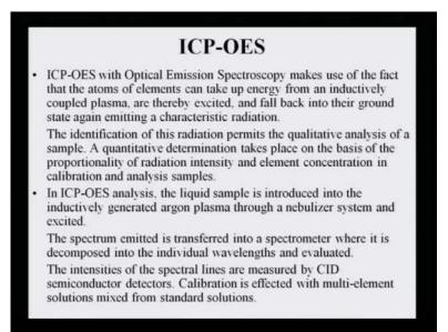
ICP-OES - ICP-OES is optical emission spectroscopy, which makes use of the fact that the atoms of elements can take up energy from an inductively coupled plasma, are thereby excited and fall back into their ground state again, emitting a characteristic radiation.
