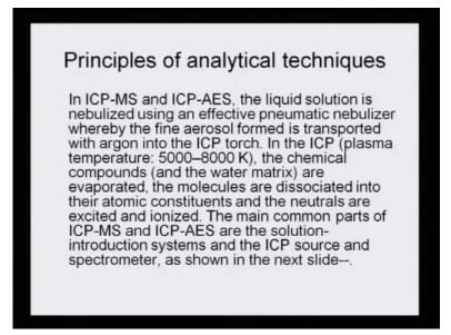
Principles of analytical techniques - in ICP-MS and ICP-AES, the liquid solution is nebulized using an effective pneumatic nebulizer whereby the fine aerosol forms is transported with argon into the ICP torch. So, instead of a peristaltic pump an on ordinary nebulizer, here there is a pneumatic nebulizer; the rest remains the same.
