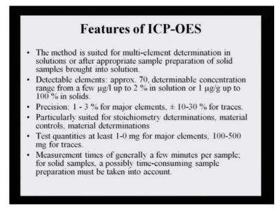
The features of ICP-OES - the method is suited for multi-element determination in solution or after appropriate sample preparation of solid samples brought into solution. So, it is both applicable to solid samples as well as appropriately dissolved samples can be prepared and multi-element determination can be carried out using ICP optical emission spectroscopy, that is, ICP-OES.
