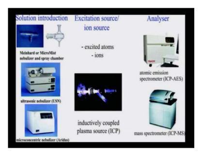
Different types of models and different types of its adaptation are required and therefore, the machine can then be used. You see, this is an ICP-MS machine; this is a simple ICP. When you have a microconcentric nebulizer, how it looks like; if it has ultrasonic nebulizer, how the machine looks like and so on and so forth.
