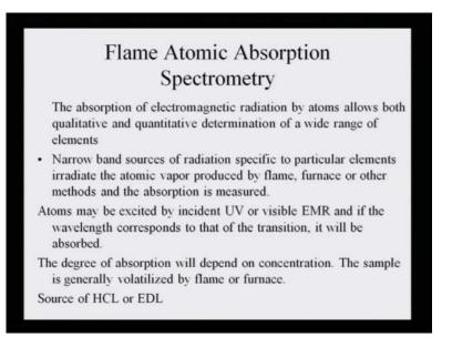
Flame atomic absorption spectrometry - the absorption of electromagnetic radiation by atoms allows both qualitative and quantitative determination of a wide range of elements. So, not only qualitative, whether it is present or absent, but also how much of it in concentration is present can be determined for a large variety of elements.
