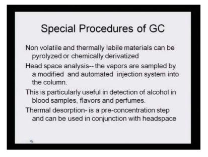
First, let us look at the injection system special procedures of GC nonvolatile and thermally labile materials can be pyrolyzed or chemically derivatized. There are now, the machine now getting into more and more specific kind of analysis and sometimes, some materials which are nonvolatile and which are also at times thermally labial which means, that the decompose at high temperature can be pyrolized or they can be turned into a derivative - we call it chemically derivatized.
