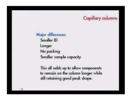
Capillary columns more emphasis has been made on capillary column because, in today's experimental conditions more and more use of capillary columns are being noticed because packed column meant for larger volume of analysis. So, the capillary column needs a special retention. Major differences in the capillary column and the packed column are that they are smaller in their internal diameter id; they are much longer in size. I said they are almost like 50 meters and they have been rolled up.
