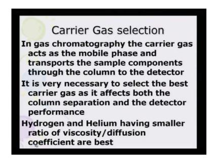
Carrier gas selection: it is a very important and a crucial decision in gas chromatography. The carrier gas acts as a mobile phase and the transports the sample components through the column to the detector. It is the main part which is you know, allowing it to move; it is very necessary to select the best carrier gas as it affects both the column separation and the detector performance.
