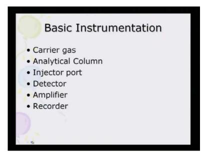
Now, these are different mode basic instrument contains carrier gas analytical column injector detector amplifier and recorder.
