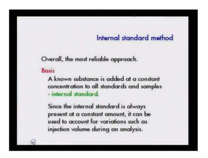
Internal standard method: overall the most reliable approach. The basis is that, a known substance or a standard is added at a constant concentration to all standards and samples and that is why it is called internal standard.
