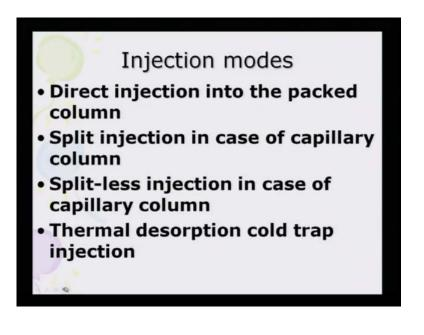
Injection mode could be direction injection into the packed columns. Split injection in the case of capillary column; split-less injection also in the case of capillary column. Thermal desorption cold trap injection which are very specific for gaseous samples.
