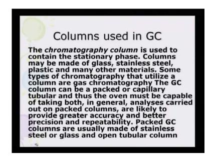
Column used in GC: the chromatography column is used to contain the stationary phase columns may be made of glass, stainless steel, plastic and many other materials. Some types of chromatography that utilize a column are gas chromatography. The GC column can be packed or capillary tubular and thus the oven must be capable of taking all the different types of columns that can be seated in that oven.
