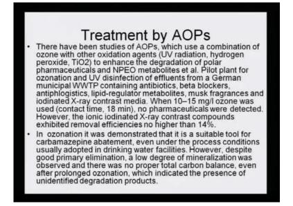
Treatment by AOPs - there have been studies of AOPs, which use a combination of ozone and other oxidative reagents UV radiation, hydrogen peroxide, titanium dioxide to enhance the degradation of polar pharmaceuticals and NEO metabolites.
