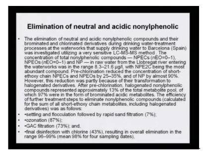
Then ozonation takes place and 87 percent purification is possible. Then, with the use of Granular Activity Charcoal, another 73 percent you know of such metabolites can be removed and final disinfection with chlorine resulting in overall elimination in the range of 96 to 99 percent can be achieved for the drinking water.
