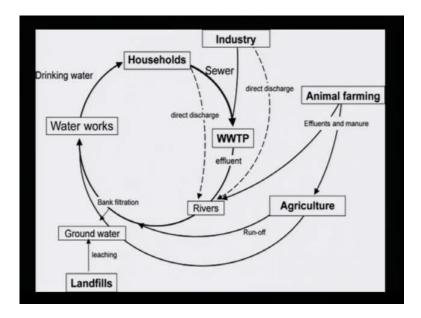
Now, if we try to look at this particular slide, we will see that, how the household water through the sewer, goes to the wastewater treatment plant and then it is then run into the rivers. The water works are supposed to be purifying and supplying the drinking water. So, that is what the water cycle looks like. Then, there are industries which make direct discharge, untreated discharge in the rivers and we have seen this example in river Ganga.
