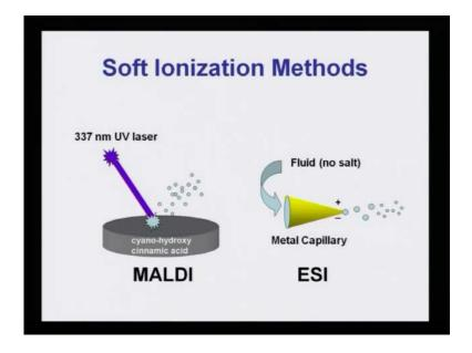
Now, what exactly happens when we talk that this is a soft method? How does the soft ionization method actually function? Now, in MALDI there is a cyano-hydroxy cinnamic acid surface, and on that, a UV laser is impacted and that creates the fragments or the ions. So, that is why it is called a soft method, because a laser beam of 337 nanometer,
