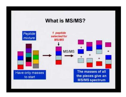
It is something like this. If I have to show you by block diagram and there is a peptide mixture, I have only masses to start with, one peptide is selected for MS/MS detection, and then slowly it breaks down into various possible fragments. The masses of all the pieces give an MS/MS spectrum. And, when all these information are correlated, then we are able to get to the actual structural determination of the peptide.
