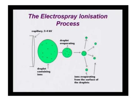
Now, the electrospray ionization process – that the droplet containing the ions is a segregate. From that, the droplet gets evaporated and the ions are spread out. So, that is where the spraying effect or the ions evaporating from the surface of the droplets actually release the ions, and that is what moves towards the detector.
