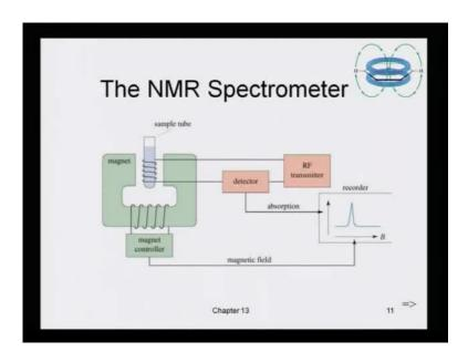
This is how the NMR spectrometer looks like. There is a huge magnet, there is a sample tube and the, there is a RF transmitter, which will create radio frequencies, there is a detector, which will be collecting the information and the detector will then, through the absorption, will go into the recorder, and the magnet actually, is controlled by a huge magnetic field. Therefore, it, this is a very simple pictorial description of an NMR spectrometer.
