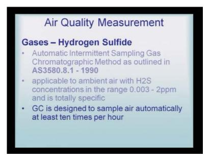
Gaseous hydrogen sulfide also, when it is in high and toxic quantity, can be a very serious air pollutant. Automated intermittent sampling gas chromatographic method, as outlined in AS3580.8.1, which was released in 1990, is the method for analysis or is the device for an analyzing the hydrogen sulfide.
