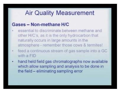
Non-methane, that is H/C, that essentially to discriminate between methane and other HCs, as it is the only hydrocarbon that naturally occurs in large amount in the atmosphere. So, you see, it is quite important to be able to analyze not only the carbon monoxides, the SOx, the NOx, and the ozone, but also sometimes, some other pollutants need to be analyzed. And therefore, there should be detecting devices to analyze the same.
