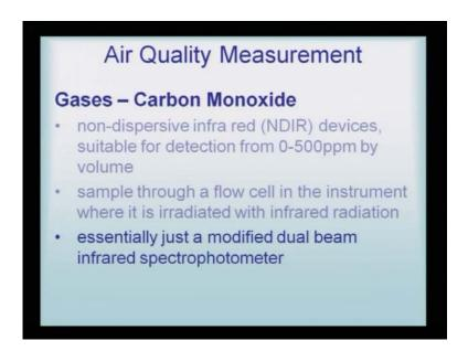
Continuing with the air quality measurement, the analysis of carbon monoxide has to be done in another very specific manner - non-dispersive infrared (NDIR) devices, are most suited for detection of 0 to 500 ppm by volume. So, this has completely new method. The SOx and the NOx could be done by UV method, but carbon monoxide requires a non-dispersive infrared device.
