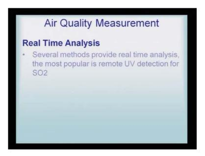
Real time analysis – several methods provide real time analysis, the most popular is the remote UV detection for sulfur dioxide. As I told you time and again, I have been telling you, that every pollutant, every chemical, needs to be treated as a special identity, and the method of determination of these are very typical and specific.
