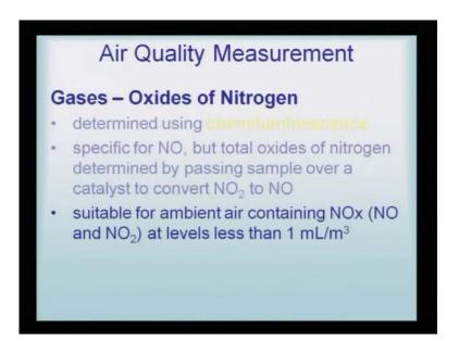
Then, gases of nitrogen, because I have been referring to this as NOX; it should be kept clearly in mind that this is more than one type of nitrogen oxide that needs to be referred.
