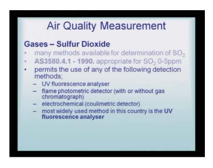
Then, comes the gaseous sampling and analysis of various other pollutants – the first one being sulfur dioxide – many methods are available for determination of sulfur dioxide; one of the method of course, is the AS3580.4.1, which was released 1990, which is most appropriate for sulfur dioxide to be analyzed between the range of 0-5 parts per million or ppm; permits the use of any of the flowing detection methods. That means, one can
