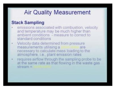
Stack sampling – emissions associated with combustion, velocity and temperature may be much higher than ambient conditions – measure to correct to the standard conditions. Now, what happens in factories? One needs to put a check on what are the emissions rates; sometimes, the combustion – if it has not taken place properly in the furnace, it will emit all kinds of bad gases and the notorious pollutants, and that needs to be checked.
