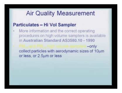
Particulate high volume sampler – more information and correct operating conditions can also been learnt from another standard, Australian standard, AS3580.10, which was released in 1990. Here, the PM 10 and the PM 2.5 high volume samplers only collect particles with aerodynamic sizes of 10 micron or less or 2.5 microns or less; recognized by PM 10 head, which looks like a cross between a flying saucer and an overgrown wok.
