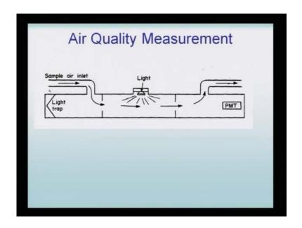
And, this is how it looks like – there is a source of light; there is a sample, an air inlet and it has a flowing path, and during the path, it is trapped and analyzed by the detector.
