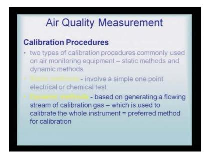
Calibration processes again have two more important things to be told. Two types of calibration procedures mainly used on air monitoring equipment are the static methods and the dynamic methods. The static method involves a simple one point electrical or chemical test. As the name suggests, you know into the air sample, some reagent may be added and just on the spot, it is kind of tested.
