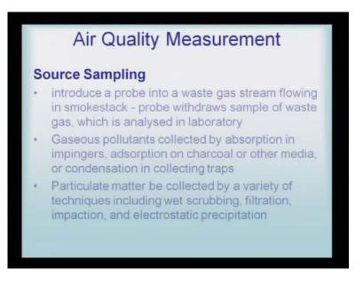
Source sampling – how does it take place? Introduce a probe into a waste gas stream flowing in smokestack – probe withdraws sample of waste gas, which is analyzed in laboratory. So, how does this take place? Introduce a probe into a waste gas stream flowing in smokestack, and then, try to probe. The probe then, withdraws the sample from the waste gas.
