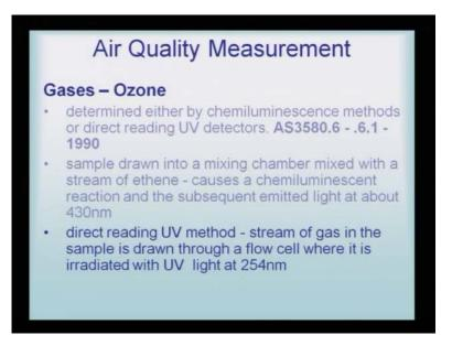
Ozone – determined either by chemiluminescence methods or direct reading by UV detectors. Sample drawn into a mixing chamber mixed with a stream of ethane – causes a chemiluminescence reaction and the subsequent emitted light at about 430 nanometer. Direct reading of UV method – stream of gas in the sample is drawn through a flow cell, where it is irradiated with UV light at 254 nanometers. So, it is a very simple UV method of analysis and it is a foolproof method of analyzing ozone.
