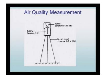
Now, this is how it looks like – there is a bottle, there is a fennel, and there is a metal stand. So, in the bottle, it is trapped and there is a gauge at the point of entry. Particulates high volume sampler – this is called a particulate high volume sampler.
