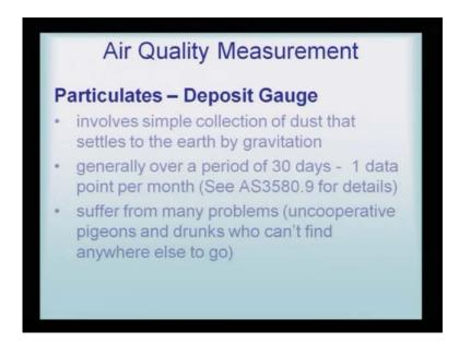
Particulates are actually measured on deposit gauge – involves simple collection of dust that settles on earth by gravitation. Generally, over a period of 30 days – a data point per month, that is, if you refer to the AS3580.9, more details can be obtained. Suffers from
