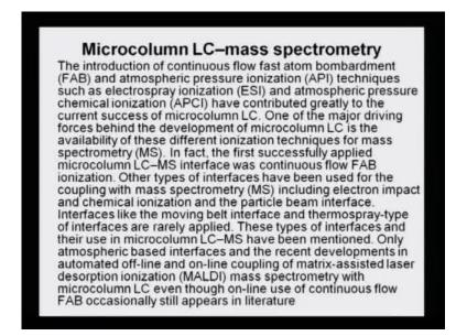
Microcolumn LC with the mass detector - that means, it is a micro column LC mass spectrometry. The introduction of continuous flow fast atom bombardment and atmospheric pressure ionization, that is, API techniques such as electro spray ionization, that is, ESI and atmospheric pressure chemical ionization (APCI) have contributed greatly to the current success of micro column LC.
