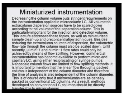
Miniaturized instrumentation - decreasing the column volume puts stringent requirements on the instrumentation applied in micro column LC. Time and again, I am repeating the word micro, which means we are making it smaller. All volumetric extra column dispersion sources have to be scaled down according to the volume of the separation column.
