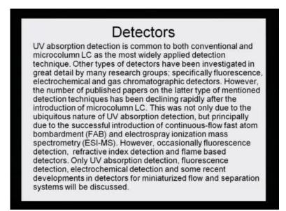
Detectors - UV absorption detection is common to both conventional and micro column LC as the most widely applied detection technique. Other types of detectors have been investigated in great details by many research groups; specifically the fluorescence, electrochemical and gas chromatographic detectors. However, the number of published papers on the latter type as mentioned in the detection techniques series, has been declining rapidly after the introduction of the micro column LC.
