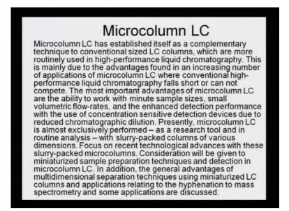
Micro column LC - micro column LC has established itself as a complementary technique to conventional sized LC columns, which are more routinely used in high-performance liquid chromatography. is mainly due to the advantages found in an increasing number of applications of micro column LC, where conventional high-performance liquid chromatography falls short or cannot compete.
