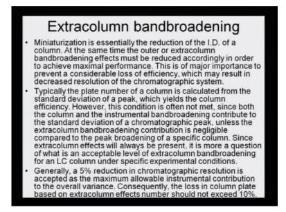
Miniaturization is essentially the reduction of the internal diameter or the I.D. of a column. At the same time, the outer or extra column band broadening effects must be reduced accordingly, in order to achieve maximum performance. This is of major importance to prevent a considerable loss of efficiency.
