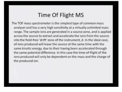
Time of flight is one of the common mass analyzer. We have talked about it in the previous class. The time of flight mass spectrometer is very special and highly sensitive, and therefore, it is one of the most latest techniques of today's mass analyzers.
