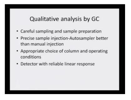
Qualitative analysis can be carried out by GC - Careful sampling and sample preparation; precise sample injection - auto sampler is better than manual injection; appropriate choice of column and operating conditions; detector with reliable linear response. Now, this particular slide requires a little more attention.
