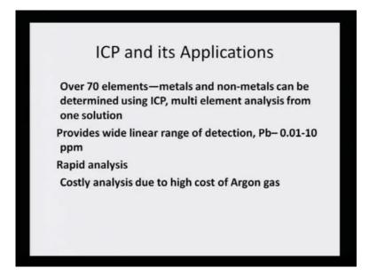
ICP and its applications - over 70 elements, metal and non-metals can be determined using ICP, multi element analysis from one solution. So, you see that their hair is a machine which can do miracle. One can just take one solution and an analyze seventy elements in one go whereas, in atomic absorption one had to analyze one by one; it was more time consuming, but there are always advantages and there are limitations.
