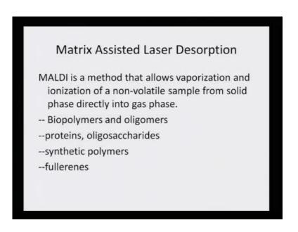
Matrix assisted laser desorption - this is a technique which is called MALDI, is a method that allows vaporization and ionization of non-volatile samples from solid phase directly into the gaseous phase. Biopolymers and oligopolymers can be analyzed by MALDI, this option method; proteins and oligosaccharides, synthetic polymers and fullerenes can be
