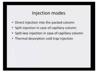
There are different injection modes also. There could be a direct injection mode on the packed column or capillary column; there could be a split injection in the case of capillary column. Why do we need a split injection? Because the entire amount need not necessarily passed through the capillary column.
