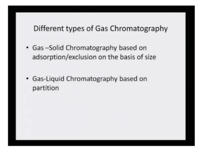
Different types of gas chromatography - there could be gas-solid chromatography based on adsorption and exclusion on the basis of the size or it could be gas-liquid chromatography based on the partitioning of these different components that I showed you in the previous line.
