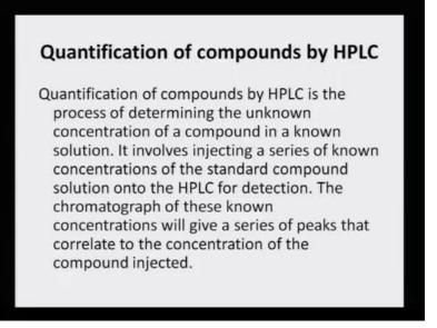
Quantification of compounds by HPLC - Quantification of compounds by HPLC is a process of determining the unknown concentration of the compound in a known solution. It involves injecting a series of known concentrations of standard compound solution onto the HPLC for detection. The chromatograph of these known concentrations will give a series of peaks that correlate to the concentration of the compound injected.
