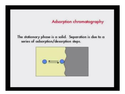
Adsorption chromatography - how it works? The stationary phase is a solid. Separation is due to a series of adsorption and desorption, adsorption and desorption, and that is how it passes on to the column.
