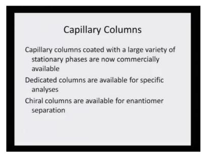
Capillary columns - capillary columns coated with large variety of stationary phases are now commercially available. Dedicated columns are available for specific analysis. Chiral columns are available for enantiomeric separation.
