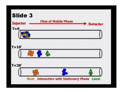
When I say with my hands that the separation is taking place like this, probably it is not so clear, but when I show it with this kind of a pictorial slide, it makes it much more clear. And here you see, in the third one, after 20 minutes of time, the components have completely separated and the one which is lowest boiling that is the green one has almost reached the other end near the detector.
