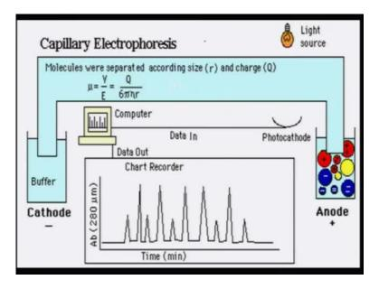
Capillary electrophoresis - if one has to see it in pictorial way, I have taken this example and would retain it for some time so that one can see how these charged ions are first separated and how they are, you know, transferred one by one to the different electrodes and they are trapped there and there is a recorder, which gives a recording to show how they are analyzed simultaneously. (Refer Slide Time: 13:42)
