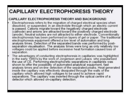
Capillary electrophoresis theory - how does it work? Capillary electrophoresis theory and its background shows that the migration of charged electrical species, when dissolved or suspended in an electrolyte through which an electrical current is passed, the cation migrates towards the negatively charged electrode, as you would know and the anions are attracted towards the positively charged electrode; neutral solutes are not attracted to either electrodes.
