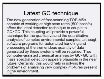
Latest GC technique - the new generation of fast scanning TOF-MS capable of working at high scan rates, that is, 500 scans per second offers the ideal detection technique to couple to GC and GC.
