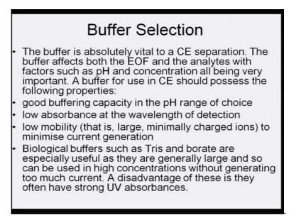
Buffer selection - that because everything is happening in this buffer solution, and so, the selection of the buffer solution is very crucial. The buffer is absolutely vital to a capillary
