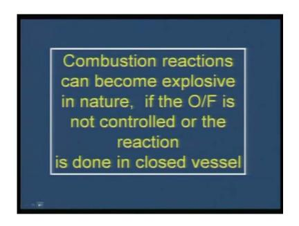
So, the point that we need to notice, combustion reactions can become explosive in nature, if the O by F ratio that is, the oxidizer to fuel combination is not controlled. And if the reaction is not done in a open vessel, this can become a potential explosive situation. Therefore, we need to be careful, to control this reaction by doing such experiments in a open vessel. Now, how to tame combustion synthesis to make material is what we are going to see.
