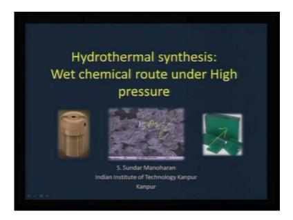
And also I have highlighted, whenever you look for Meta stable phases or unusual oxidation states in oxides, you can always resort to a very, very important approach that is hydro thermal. And I have also shown in this view graph, these are beautiful crystals of CrO2 which is used in magnetic recording industry, and how gems can also be made selectively using hydro thermal condition.
