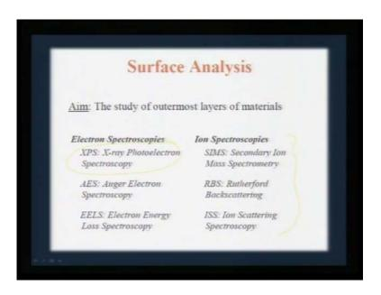
And we also looked at other surface analysis techniques which are there, I could not deal with these techniques ion spectroscopies in detail for want of time. But, we have looked more carefully into another technique that is XPS, X-ray photo electron spectroscopy.
