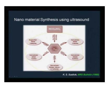
And through this ultra sound effect, we can make a host of nano materials which can be rendered in different form, either as a sulphide or as a oxide or as a support on a catalyst surface. We can realize this is in many forms provided, we start with the right combination and conditions.
