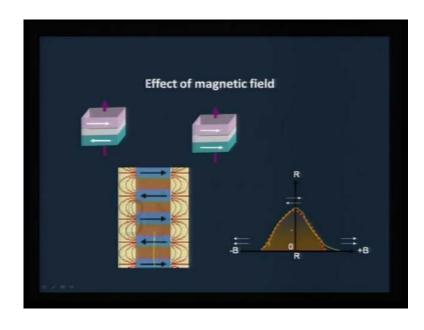
And also I have highlighted to you, how this compounds the multi layers are useful in rotating the magnetic alignment. So, with the magnetic field and without the magnetic field, how a anti ferromagnetically aligned material gets ferromagnetically aligned in a one direction; as a result you see a drop in resistance as a function of field.
