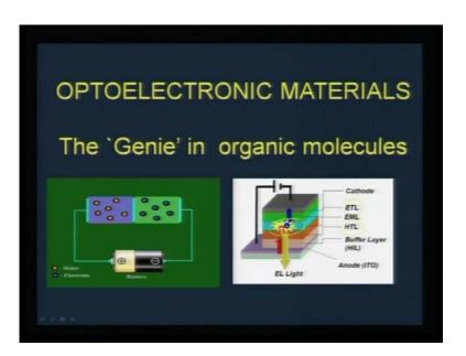
And we understood from couple of lectures on organic photonics, how this organic molecules can be used for oled applications. One such important example is the emissive layer which is very much responsible for tuning color in organic LED's, and what is the role of the whole transport layer, what is the role of electron transport layer? And how materials synthesis is very important in designing different molecules.
