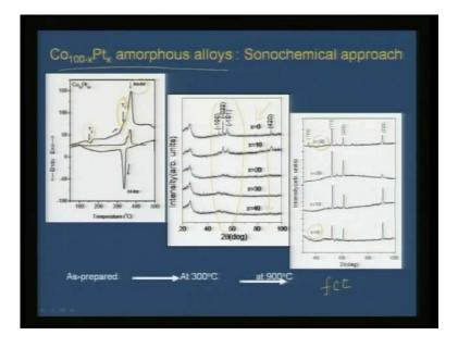
If you take the cobalt platinum amorphous alloys that we have prepared using sonochemical approach, you can see the phase transformation that is occurring. If you do the DSC curve for cobalt platinum, the first peak what you see here is the glass transition temperature; and this amorphous alloy is getting crystallized somewhere around 350 degree C. So, if you want to study this in amorphous form, you should always restrict your temperature for treating these particles well below 300.
