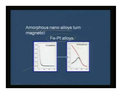
Another interesting alloy is ion platinum nano alloy, we can prepare it in amorphous nano form. But, there are interesting features that we see in ion platinum nano alloys, this is the resistivity curve for a typical ion platinum nano alloy prepared by sonochemistry, where you can see a crystalline one shows a resistivity curve like this. And amorphous curve actually shows the magnetic transition in a peculiar form.
