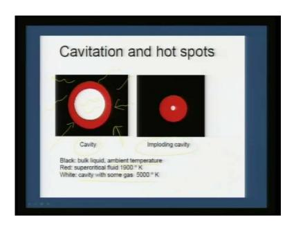
Now, cavitation and hot spots can bring about lot of issues or data's that are per se very meaningful, you see the cavity here and you see a imploding cavity here and the black region is nothing but your bulk liquid that is at ambient temperature. Now, if you actually proceed towards the bubble that temperature zone, the red one is nothing but your supercritical fluid which can even achieve temperature up to 1900 Kelvin compared to the local areas.
