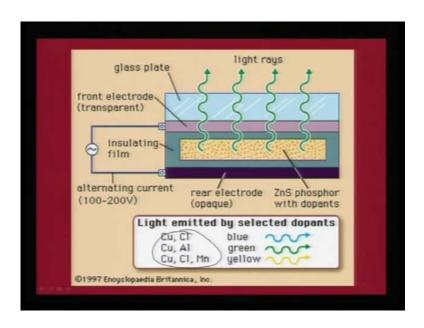
This is how the current induced photoluminescence occurs in a typical phosphor, where depending on the dopant and co-dopant, you can actually get the light output from this displays.
