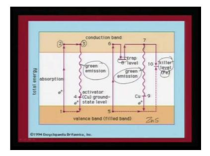
And lastly on the mechanism of how this zinc sulphide based phosphors operate, there are two, three things that can be dominant. One is the electrons are excited to from state 1 to state 2 that is the conduction band, and this can dwell in the conduction band for a short span. And then this can give out green emission, and come back to the copper ground state level and then this can return back to the ground state, so this is one process.
