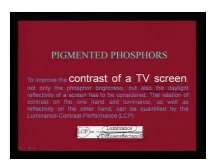
Now, when I talk about the contrast of a TV screen, we should understand the contrast is nothing but the luminescence contrast performance, this is defined as a ratio of your luminescence versus diffused reflectance. Diffused reflectance is actually coming from the stray radiation to improve the contrast of a TV screen, not only the phosphor brightness is important, just because it glows bright does not make it a good candidate.
