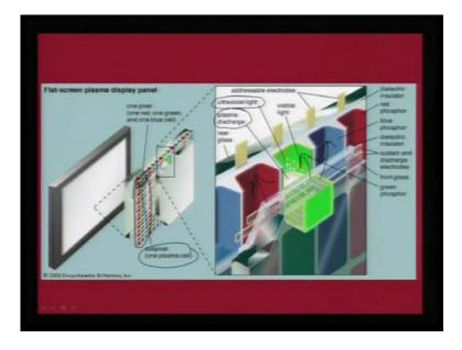
And as you would see, the display mechanism is quite different compared to the CRT applications, and in this case what you see is a plasma discharge. And this plasma discharged is actually brought about by the UV light, and once UV light is generated in the back panel that UV light will shine on the respective ones red, green and blue. And as a result you will get plasma which is generated that will account for the emission of full
