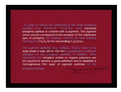
And in order to reduce the reflectivity of the white phosphor powder for example, these are all candidates for white phosphor. Each phosphor particle is covered with the pigment for example, cobalt aluminate is a good pigment for blue emitting zinc sulphide, which is doped with silver and aluminium. Similarly, you can use iron oxide it could be alpha iron oxide powder, which is actually used to control the refractivity as far as the red emitting yttria compounds are concerned.
