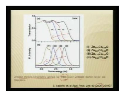
And if that is a case then what happens to the bandage, and to the PL you can see here in this case 30 percent cadmium, when you dope then it is shifting to a lower band gap. And the absorption also shifts to the lower band gap, so with increase in cadmium you can push this to a lower band gap emission. So, this is been done by MBE grown zinc cadmium oxide films, and this is reported in a PL in year 2006, so one can use MBE technique for making such hetero structures.
