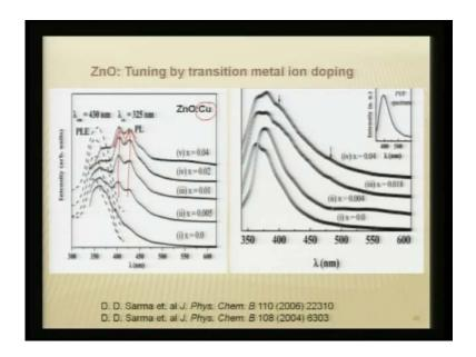
We can also try to alloy it by doping it with copper, and in this case you can see how the PL varies, the maxima shifts towards the red and PL also changes considerably with copper doping.
