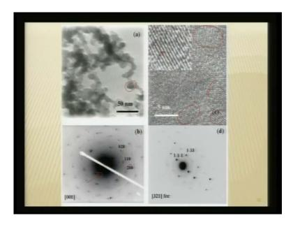
And this is the viewgraph of how the zinc sulphide, doped cadmium sulphide nano particles are and you can clearly see that these are all the embedded particles. And they clearly shows the crystallinity, and the lattice planer spacing's are specific to the zinc concentration. And this is your SAD pattern showing that these are crystalline, and we can index that to specific planes.
