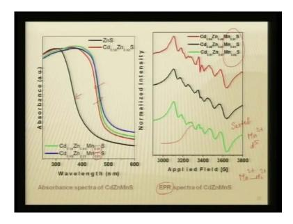
If you look at the absorption spectra, you can see that this is the zinc sulphide band gap and this is your cadmium sulphide band gap. And the moment you try to dope with manganese 1 percent in cadmium rich situation you can see that the bandage is immediately shifting to red. So, even with little incorporation of manganese it is very sensitive, so you can push this to higher band gap and how do we know that manganese is clearly doped in all these concentrations.
