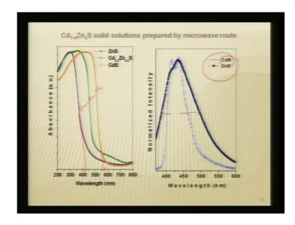
Now, when we look at the absorption spectra and the PL spectra, one can clearly understand how we can alloy this compound. And if alloying is rally true, then it has to show in the optical bandage, cadmium sulphide as I told you is low band gap material compared to zinc sulphide. So, if you actually dope cadmium sulphide with zinc, immediately you will see the shift in the absorption H, so typically you can see say from 550 it comes down to nearly 420 nanometers.
