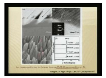
And this is the viewgraph of your zinc magnesium oxide nano needles, which are grown on silicon, you can see these are the grown needles shaped structures of this zinc magnesium oxide that you can grow. And they clearly show the lattice fringes which is typical of the zinc magnesium oxide.
