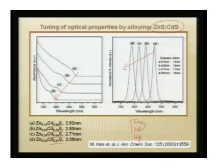
Now, another example of alloying that we have seen in the literature is that of zinc sulphide, cadmium sulphide this is not the quantum confinement issue, but this is another
