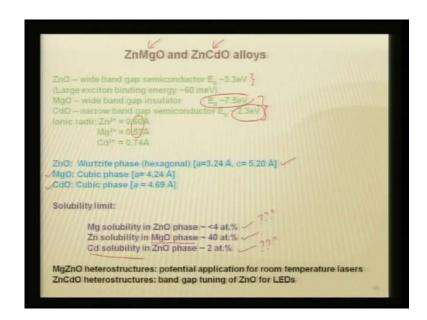
Zinc oxide is very interesting because it is used as a u V sensor, now if you want to alloy it you can try to do that either with manganese or you can try to do that with cadmium doping. So, typically the zinc oxide band gap is 3.3 E v, but you can actually dope it with the magnesium and cadmium, magnesium is a do pant which has a very high band gap that is 7.5, it is called a white band gap insulator. Now, cadmium sulphide is a low band gap stuff, so this is having 2.3.
