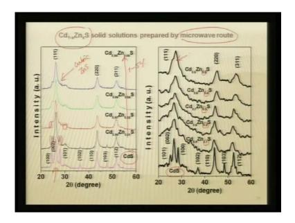
Let us take the microwave route and take specific example of cadmium sulphide which is doped with zinc. So, cadmiums if you keep on increasing from say, 1 to 5 percent of zinc you can clearly say even with the such low doping concentration, this is your cadmium sulphide typical hexagonal structure. And once you start doping with zinc, you can see that these x ray peaks are slowly coming down, and they fade and immediately transforms into a cubic phase which is typical of zinc sulphide.
