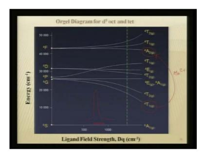
The emission that is mainly responsible for this 600 nanometer emission comes from the manganese 2 plus concentration, and this is mainly because of the 4 T 1 g to 4 A to excitation. As a result you get this pronounced 600 nanometer peak that is coming, so if you see 600 nanometer peak it is purely because of the co activator that is responsible which is nothing, but your manganese ion. So, manganese two plus will induce such a selective emission.
